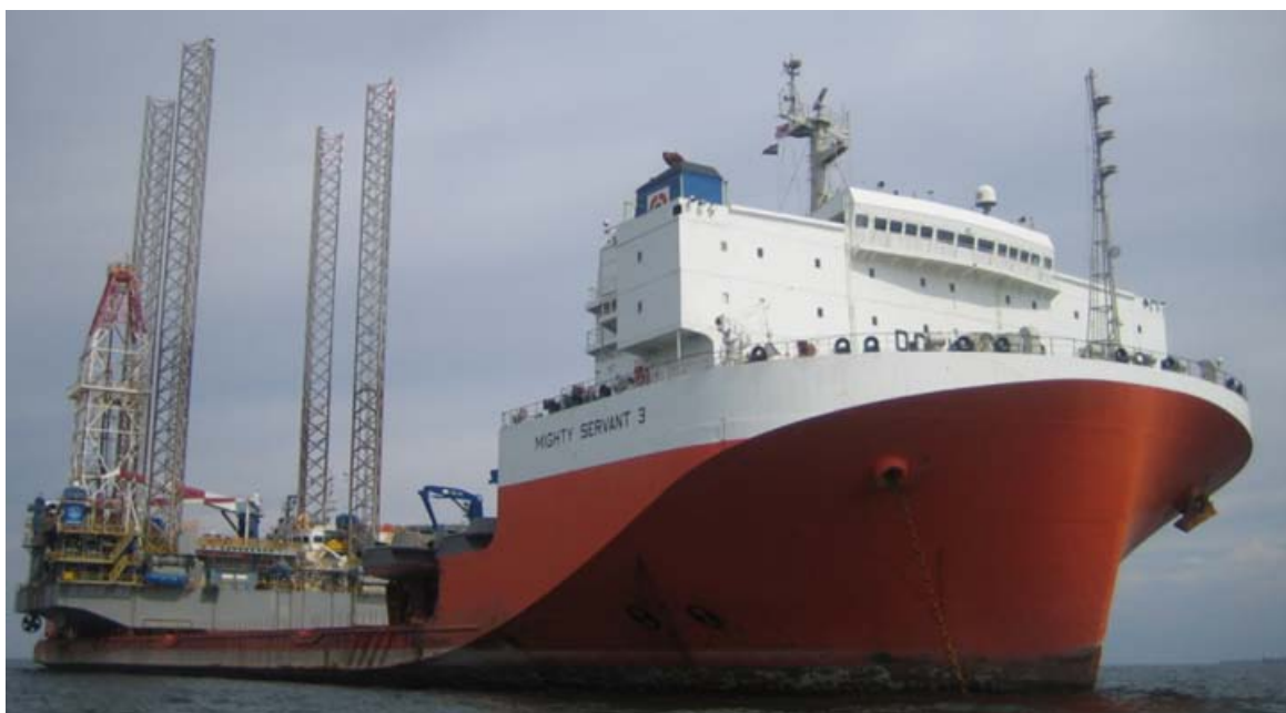
The MIGHTY SERVANT 3 seen off Labuan, Malaysia loaded with the multi purpose jack-up rig " BIMA " and two tugs. Photo : André Korver (c)
