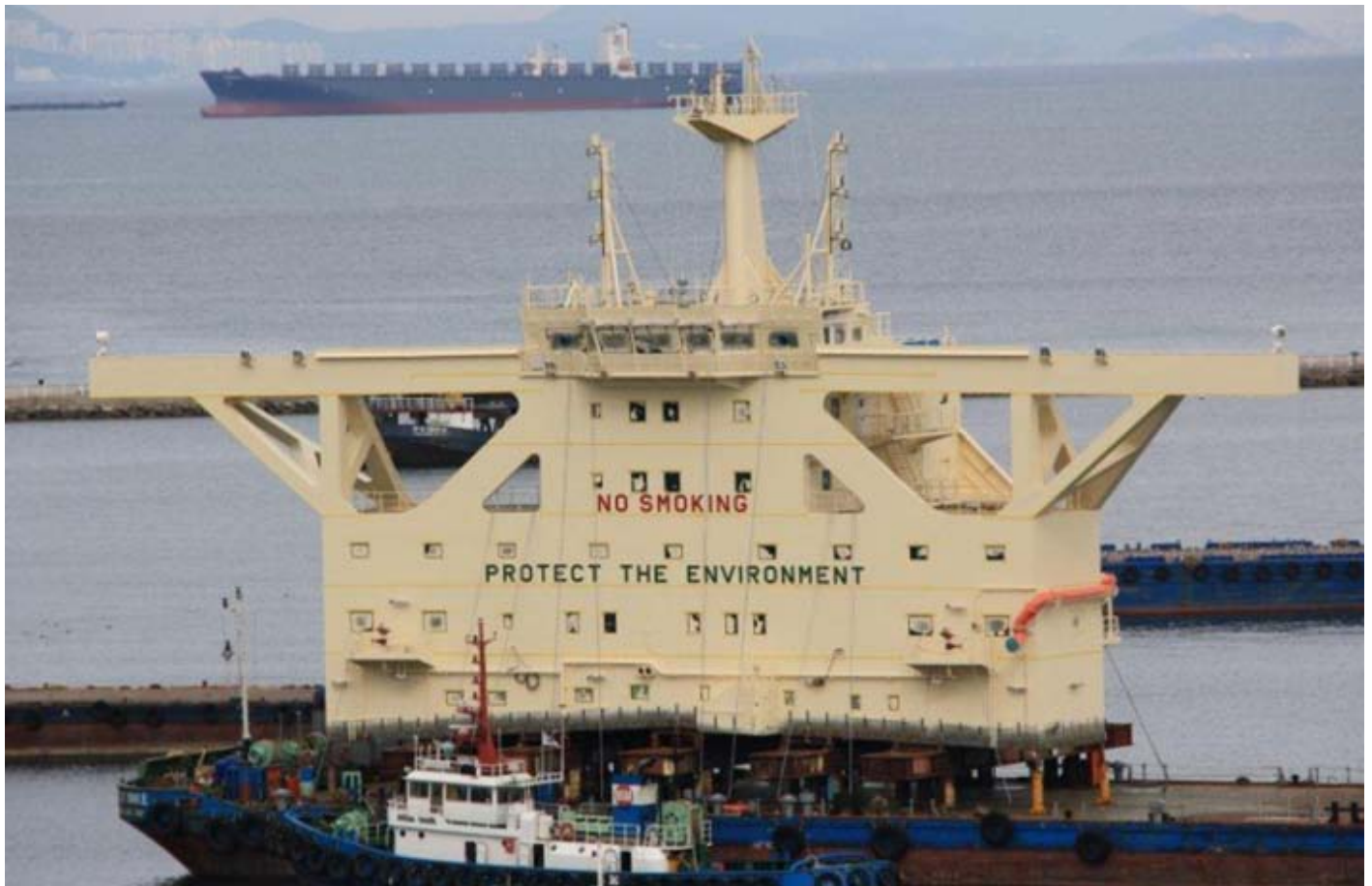
New superstructure for a tanker under construction at the DSME shipyard in Geoje (South Korea)
