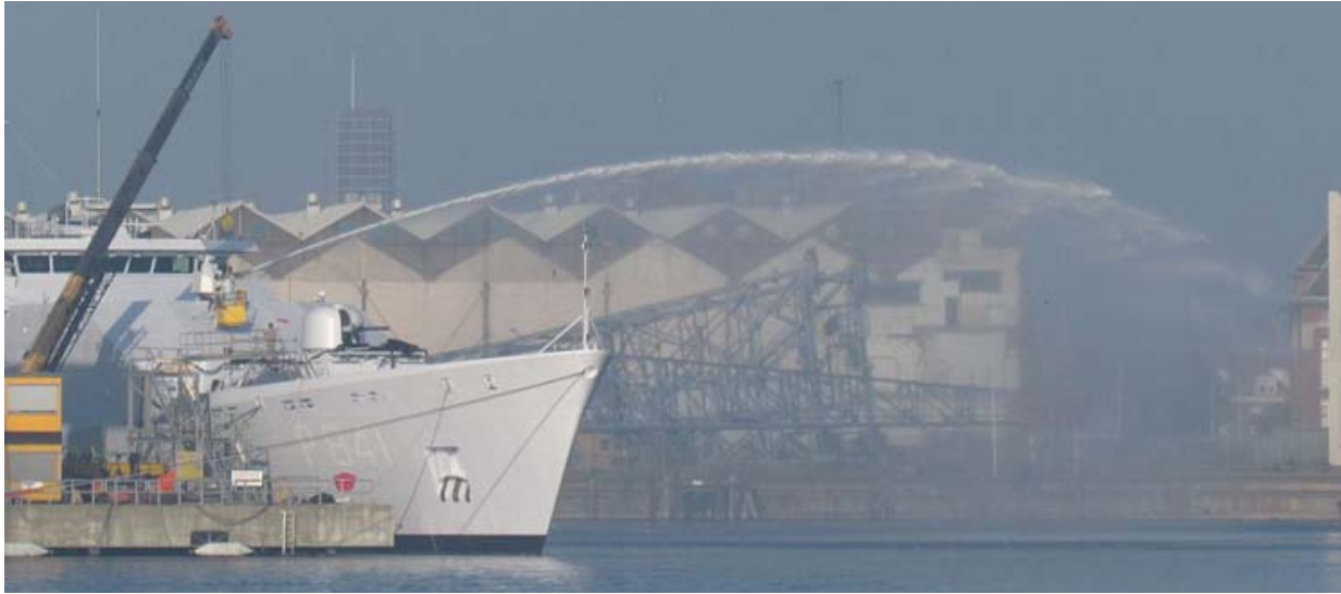
The newbuilding corvette P 841 ZEELAND seen during Fire Fighting tests at the builders Damen-De Schelde in Vlissingen - Photo : Willem Kruit ©
