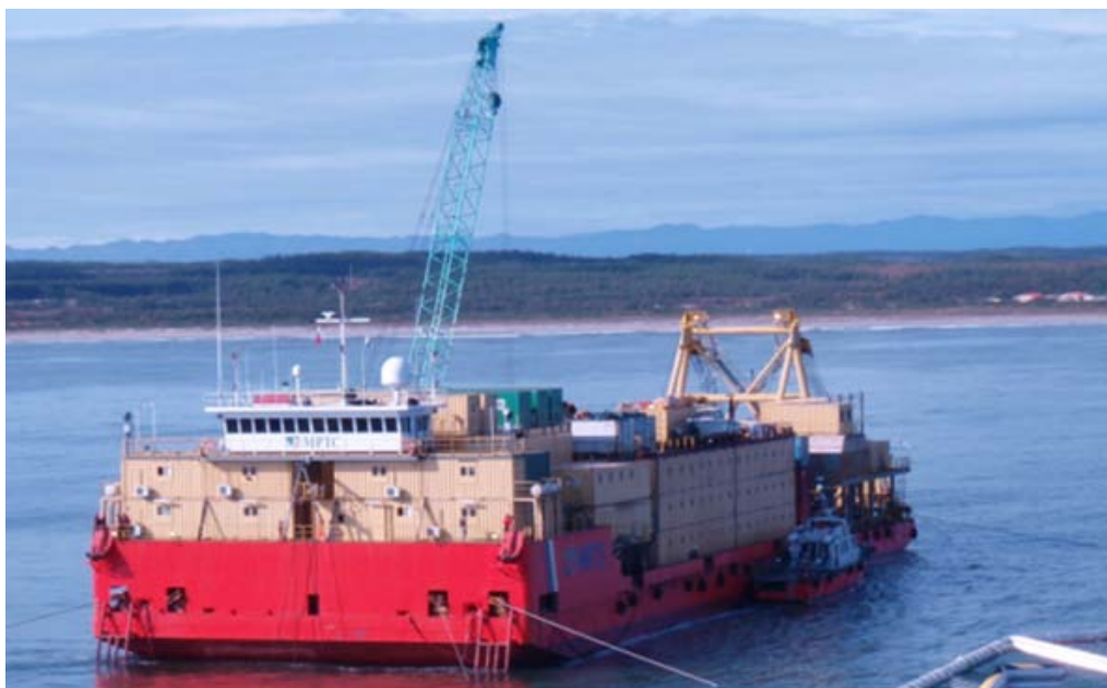
The MRTS PLB Nebula in the process of the 4 inch pipeline beach pull of the Sakhalin coast in the Kirinskoye field.
