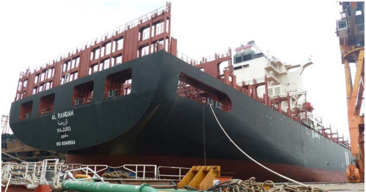
The AL RAWDAH seen in drydock at Jurong Shipyard in Singapore where a part of the ships bottom is getting replaced after the grounding off Batam last July - Photo's : E.Knisp ©
