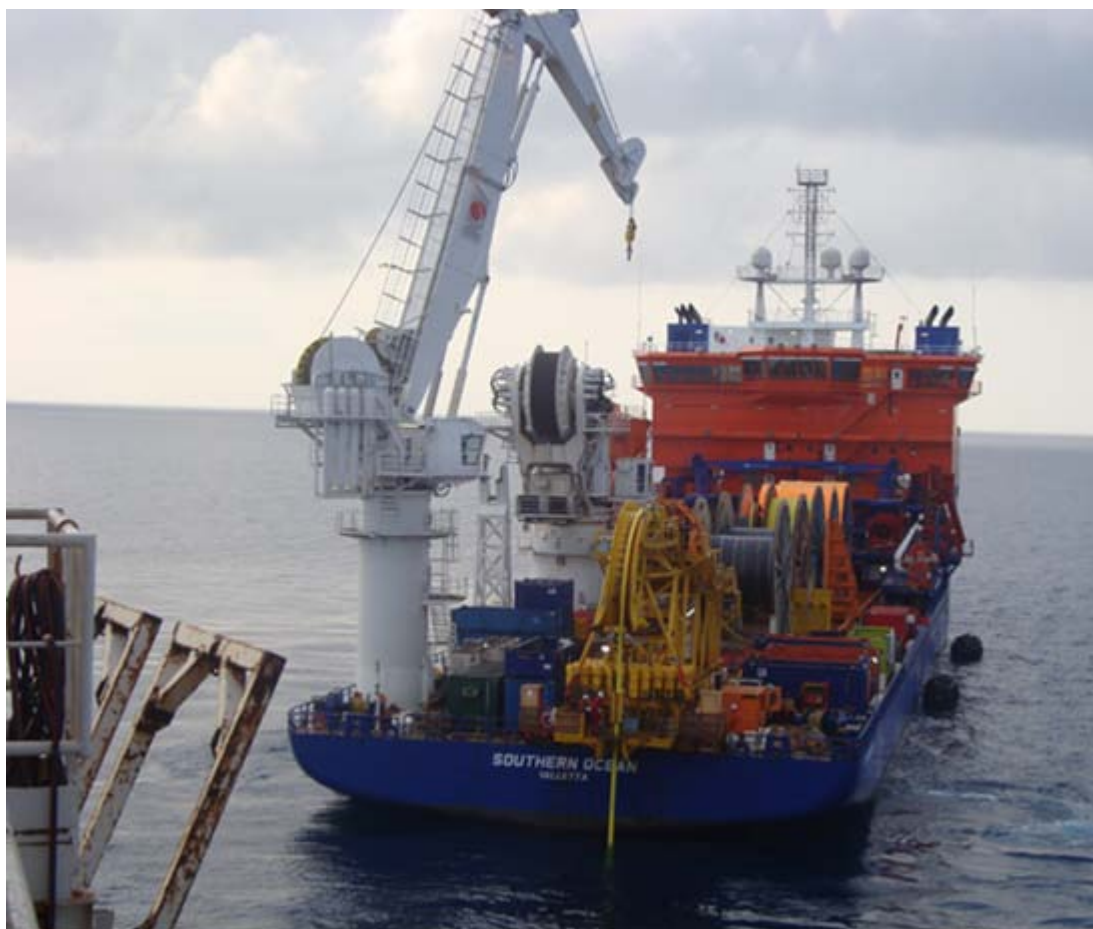
Above seen the ISV Southern Ocean installing the last of 6 risers and umbilicals for the FPSO Glas Dowl at the Kitan Field, East Timor Sea. Photo : Grant Webb ©
