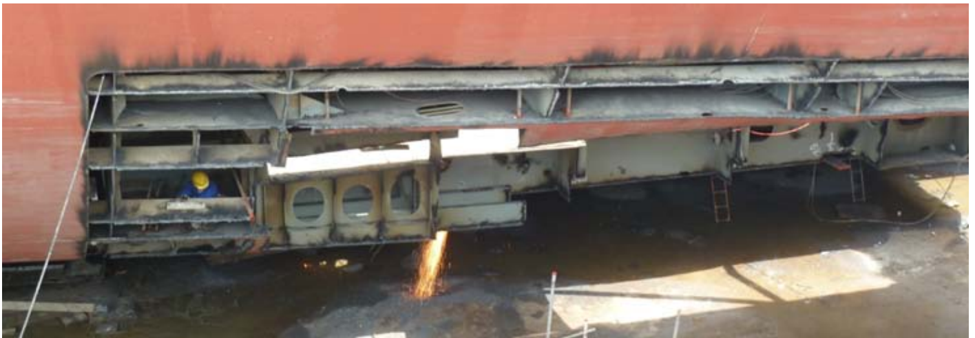
The AL RAWDAH seen in drydock at Jurong Shipyard in Singapore where a part of the ships bottom is getting replaced after the grounding off Batam last July - Photo's : E.Knisp ©
