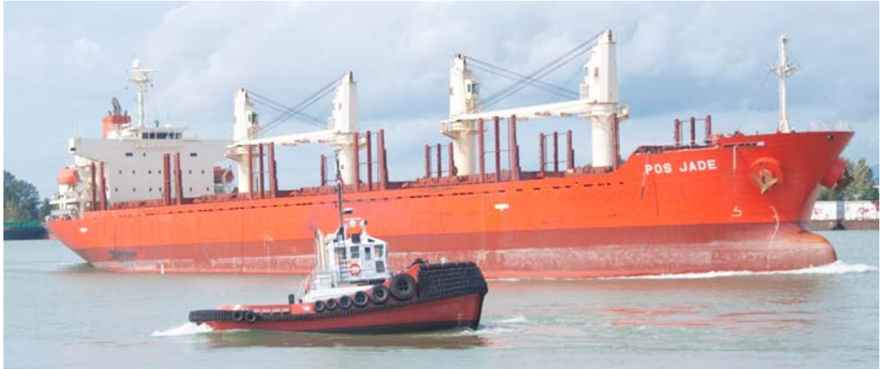
Sampson Tug Boats' new 3200 HP ship-docking tug Shuswap on the Fraser River in British Columbia. The log ship POS Jade is inbound to the Fraser Surrey docks. The Shuswap (59 x 28'3") was launched last May from the Sylte Shipyard at Maple Ridge to a Al McIlwain design. The 176x30-meter POS Jade is Japanese registered and built in 2006. Photo : Alan Haig-Brown ©
