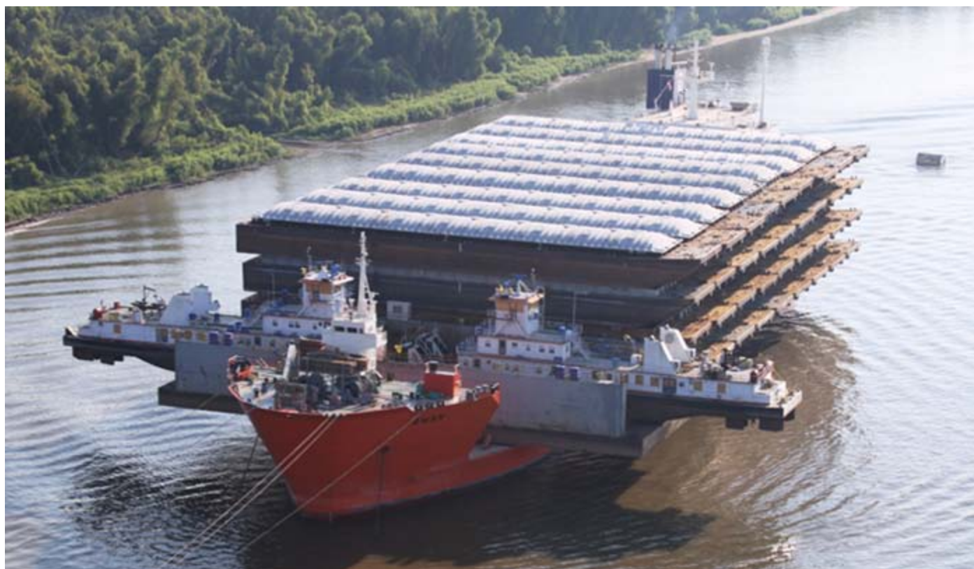
Above seen Dockwise SWAN loaded with 36 barges, 2 pusher tugs and 1 drydock in Argentina, the loaded equipment owned by NAVIOS SOUTH AMERICAN LOGISTICS, will be used to transport iron ore from southwest Brazil to the River Plate - Photo : Jan Kok – Samstrans Maritima ©
