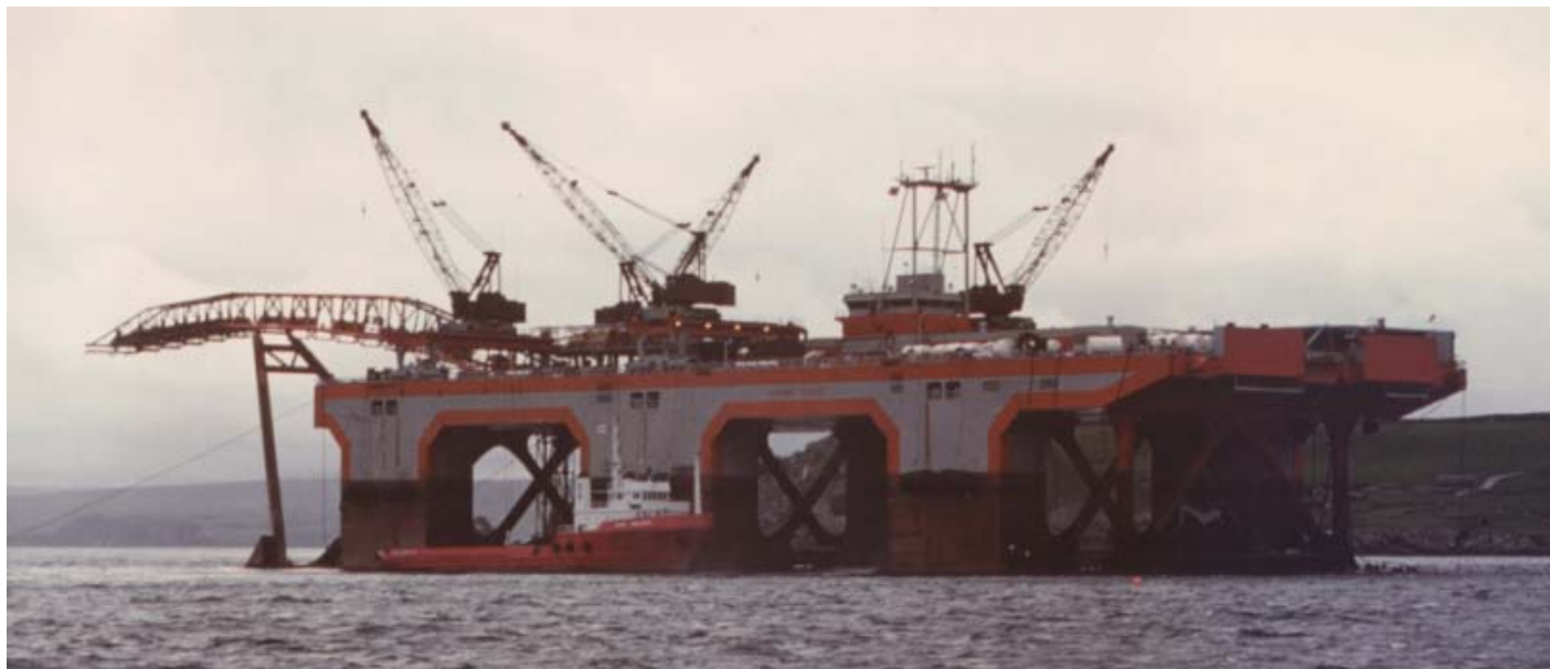
The semi-submersible pipelayer VIKING PIPER in the Bressay Sound off Lerwick (Shetlands) during final sea trials in 1976. The vessel is built by Gusto in Schiedam. Today she is owned by Saipem and is named Castoro 7 (see Shipping News Clippings 254 and 255 ) Photo : Bart J. Groeneveld ©.
