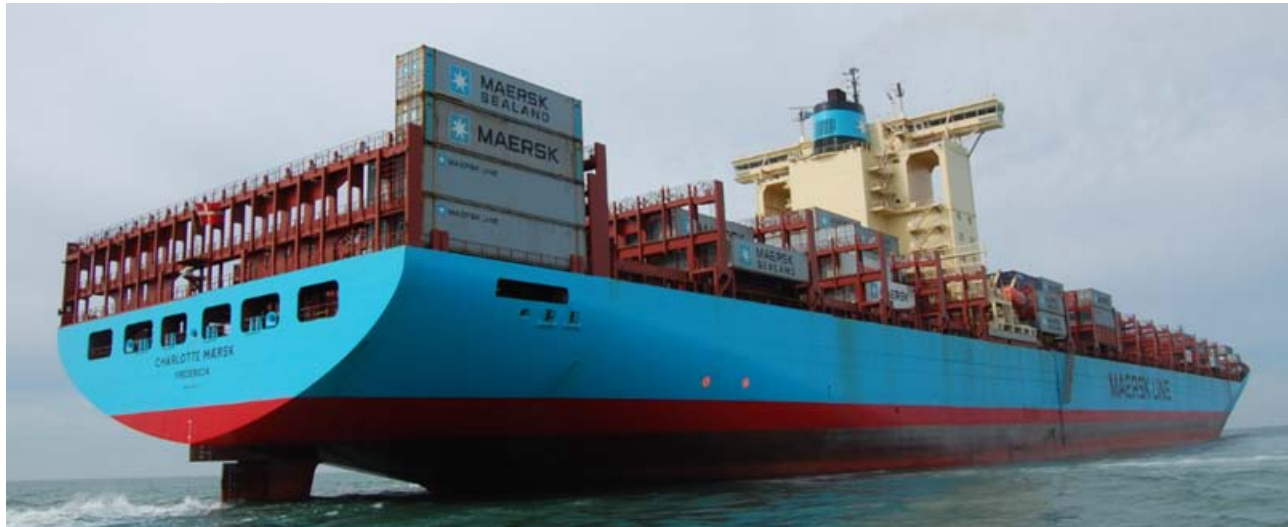
The CHARLOTTE MAERSK just completed the extension of the superstructure in China as reported earlier in the newsclippings and arrived for the first time in Rotterdam with the higher superstructure - Photo : Rik van Marle ©
