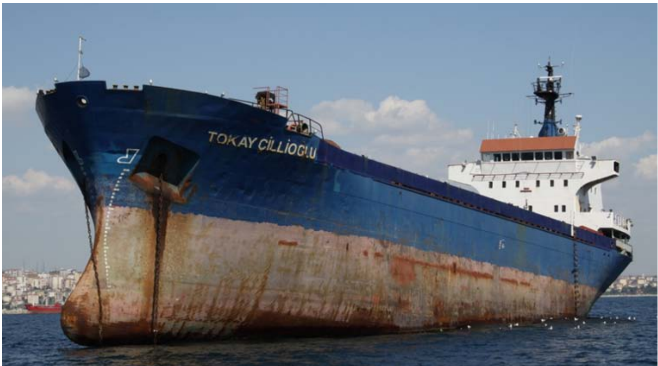
Once Spliethoff's SNOEKGRACHT the TOKAY CILLIOGLU has been laid-up off Tuzla for several years during which time her condition has deteriorated. At some point since September 2010 her cranes and foremast have been removed. - Photo : Simon Smith ©
