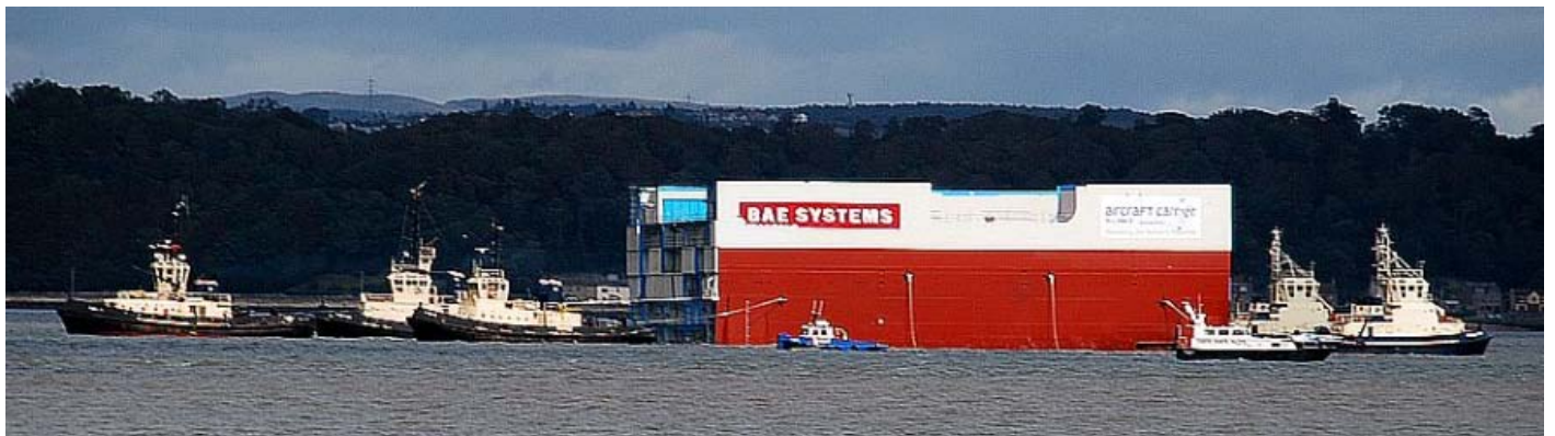
The lower midships section on the new Royal Navy Aircraft Carrier has just been floated off the barge which brought it from the River Clyde. The operation took place of Blackness Castle on the River Forth on August 30th. The attending tugs are Fidra , Seal-Carr & Oxcar of Forth Estuary Towage, plus the Svitzer tugs Cleveland Cross & Forth .
