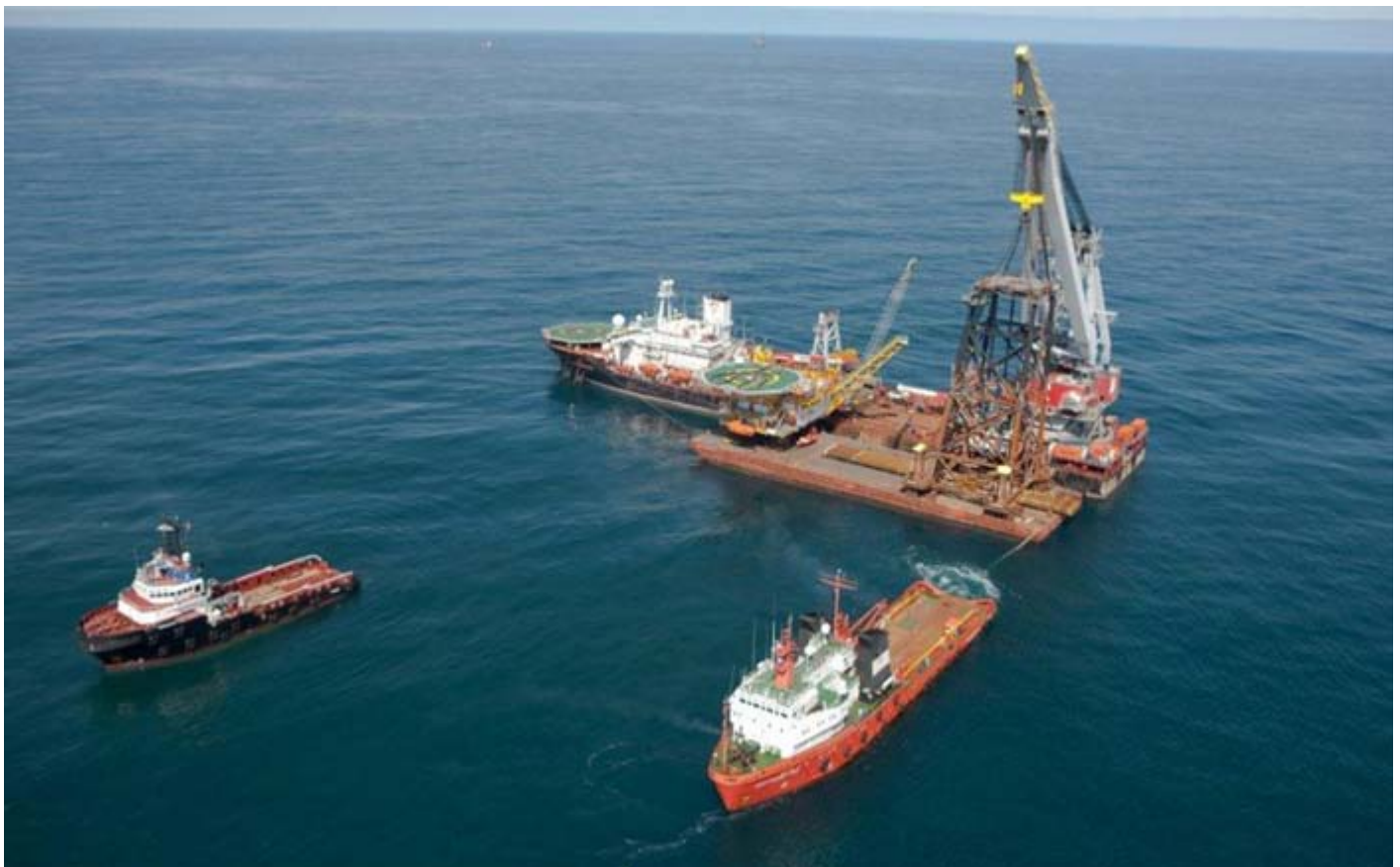
The STANISLAV YUDIN seen installing a jacket at the Wingate field - Photo : Wintershall / Aerolin
