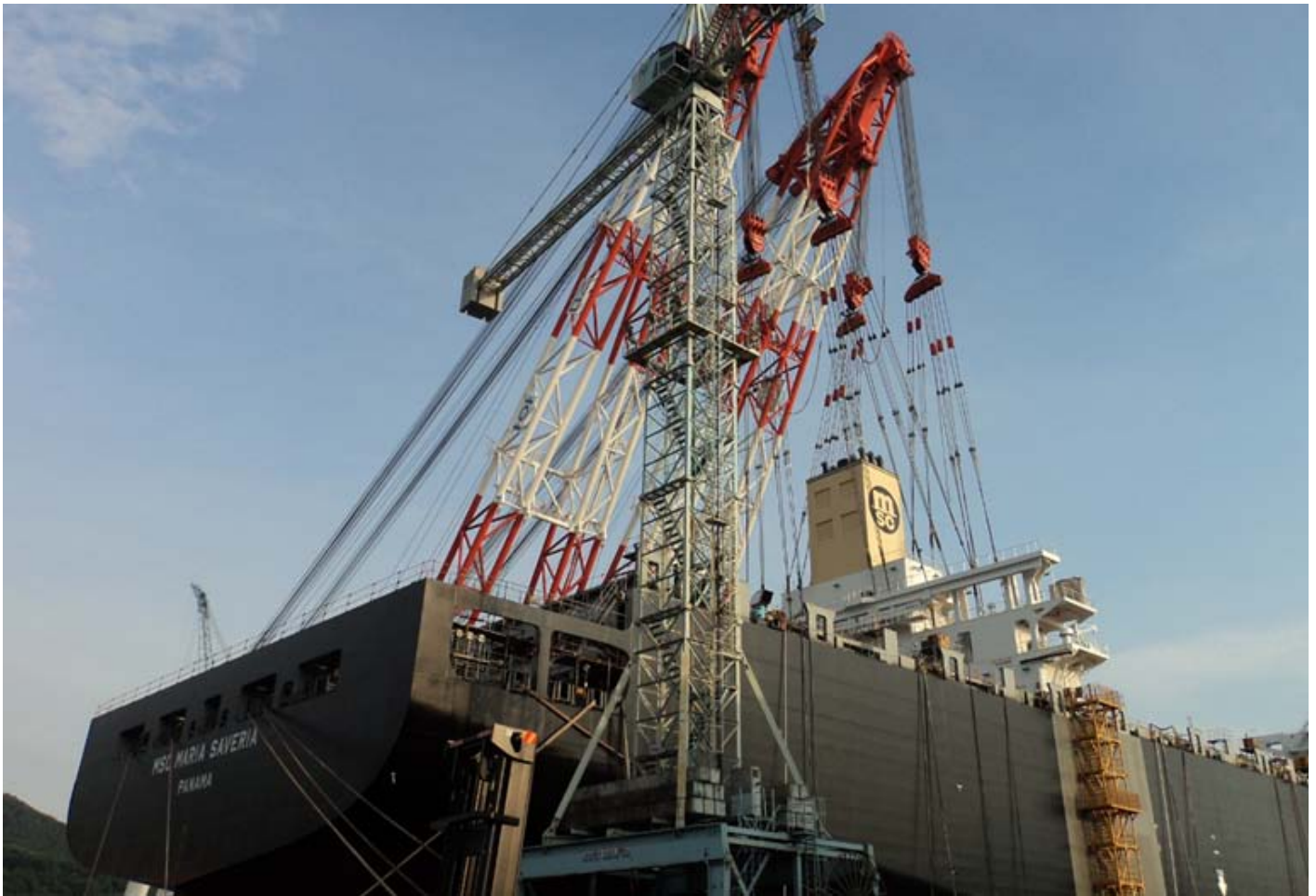
The aft superstructure of the MSC MARIA SAVERIA seen getting installed at the STX yard in Jinhae, South Korea. Photo : Bjorn de Groot ©
