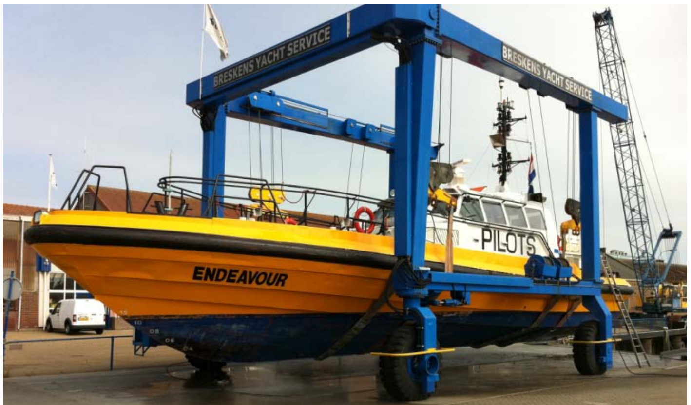
The Dutch pilot tender ENDEAVOUR seen "dry" at the Breskens Yacht Service in Breskens for hull cleaning Photo : Jamie Reurink (c)
