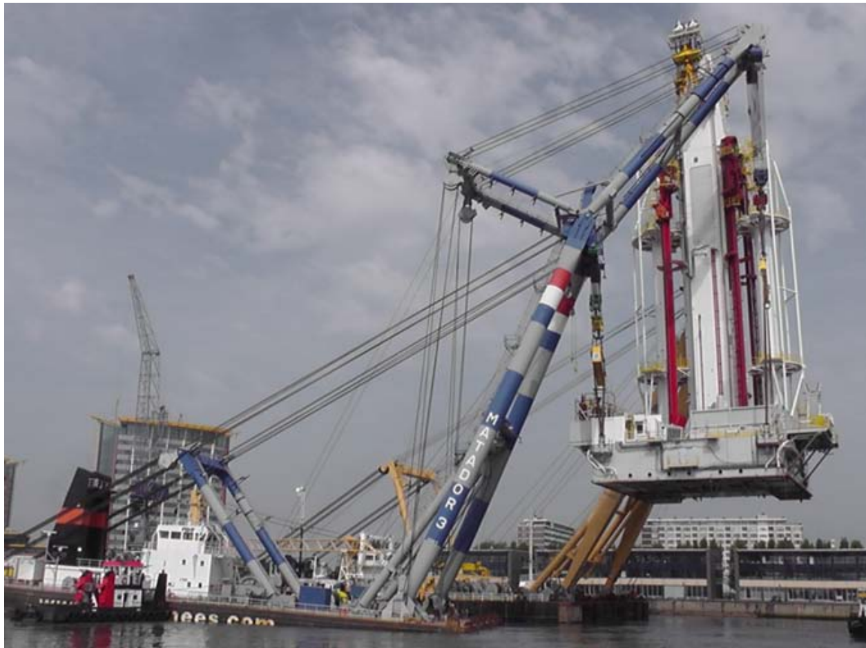
Matador 3 and Taklift 4 during loadout of drillingtower section of approx 2400ton at Huisman Yard, Schiedam . Photo : Jeroen Mooyweer (c)
