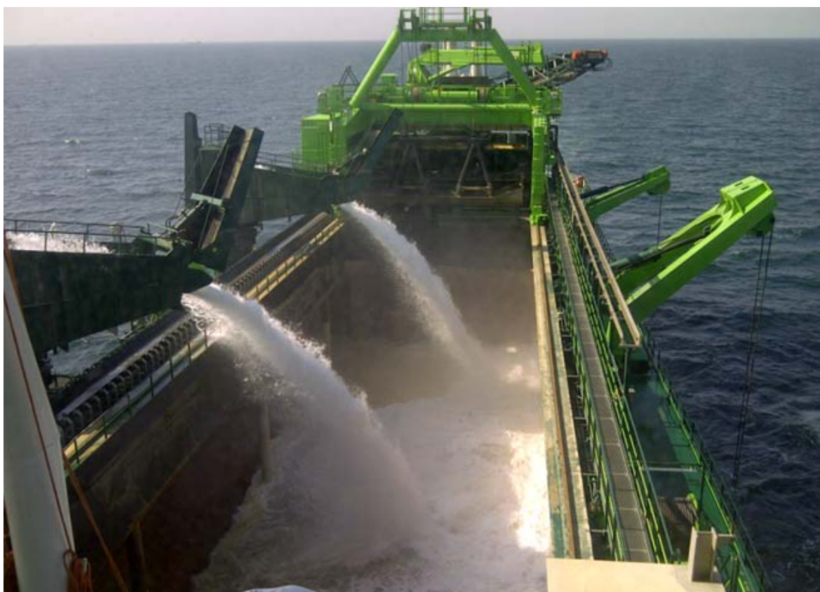
The IHC build VICTOR HORTA during hopper flushing on the way to Denmark. - Photo : Cees de Vries ©
