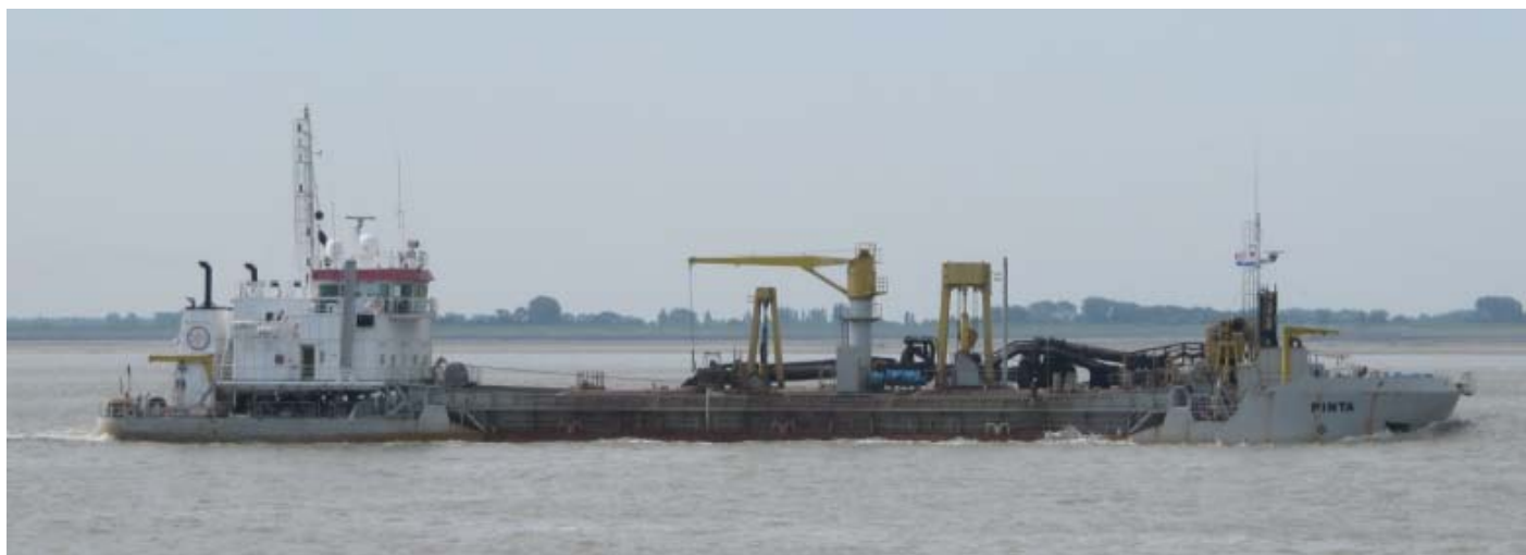
The split hopper dredger Pinta (originally designed as split hopper barge at Vuyk Rotterdam www.vuykrotterdam.com ) seen at the Westerscheldt river sailing to her discharge location. The vessel is busy with dredging activities at the river near Hansweert. - Photo : Gijsbert Jacobse ©
