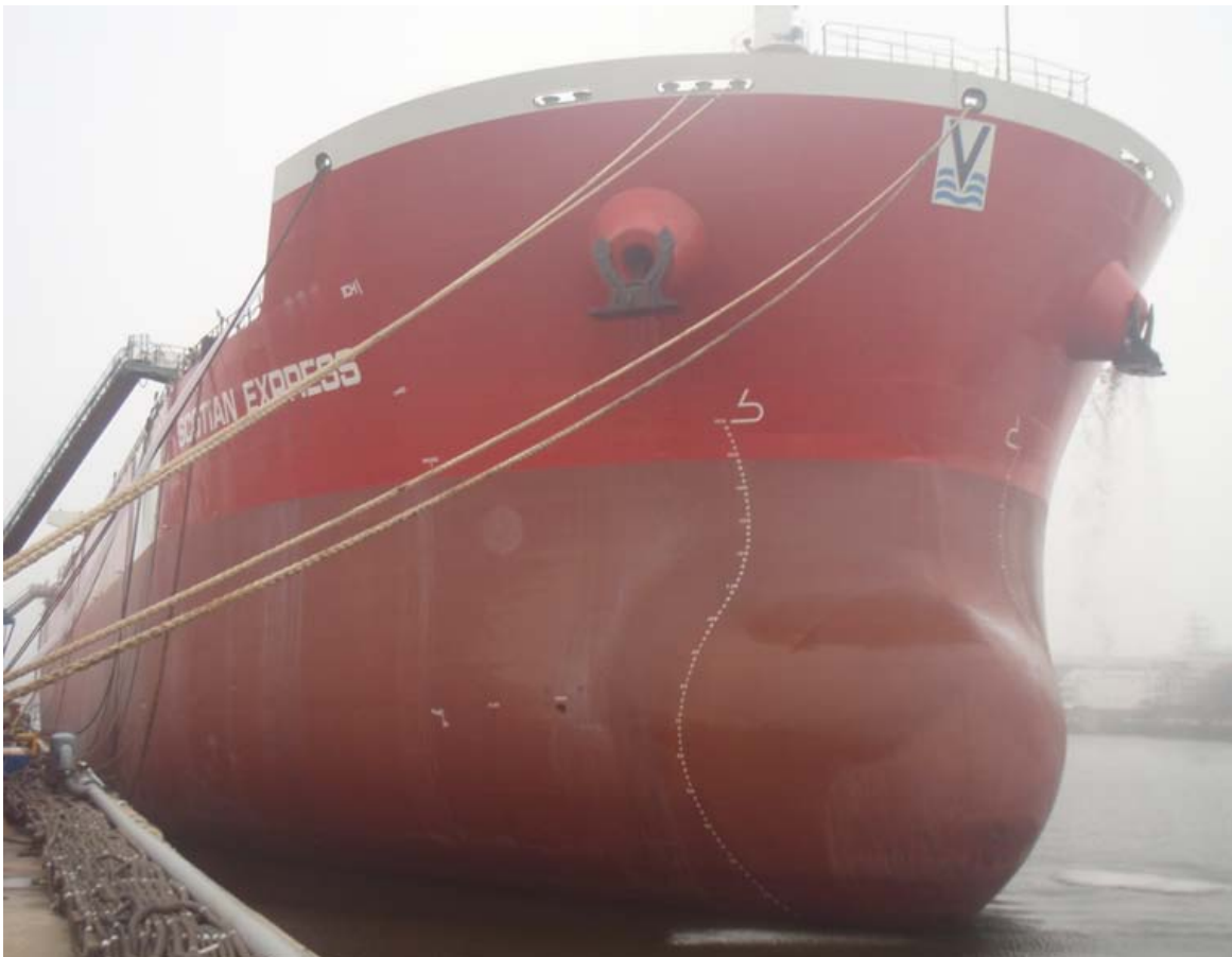
Above seen at the Cosco Dalian Shipyard a newbuilding with hull number 354 (Noble Shipping) and below a newbuilding for Vroon (Breskens – The Netherlands) the post Panamax bulk carrier SCOTIAN EXPRESS seen fitting out. The 51,209 GRT SCOTIAN EXPRESS is having a length of 229 mtr and beam of 38 mtr, and is powered by 1 MAN – B&W 6S60MC main engine of 12,240 kW for a top speed 13.7 knots - Photo's : Clemens Smits ©
