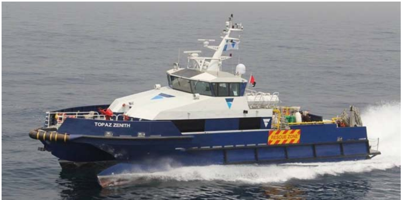
The TOPAZ ZENITH seen during trails where the crewboat reached a speed of 32 knots – Photo : Topaz marine
