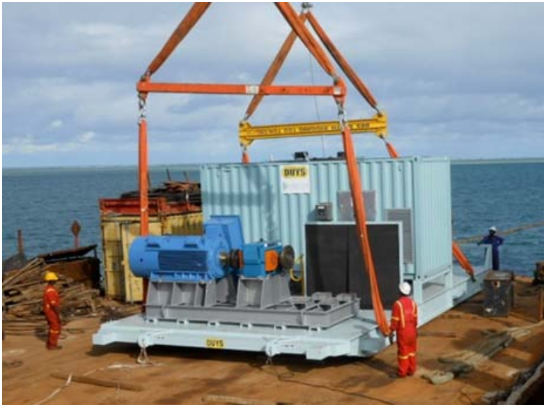
Offshore discharging of Malfamede Island, Mozambique and beach landing in MOMA of mining equipment by COMARCO using the Exposed Beach Operating System.
