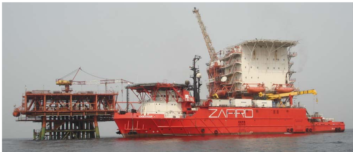
Above seen the DSV Endeavour (ex. Poseidon Endeavour ) working in Nigeria , replacing anodes at a platform with air and saturation divers. Photo : Capt. Bouke van Neutegem - Master DSV Endeavour ©
