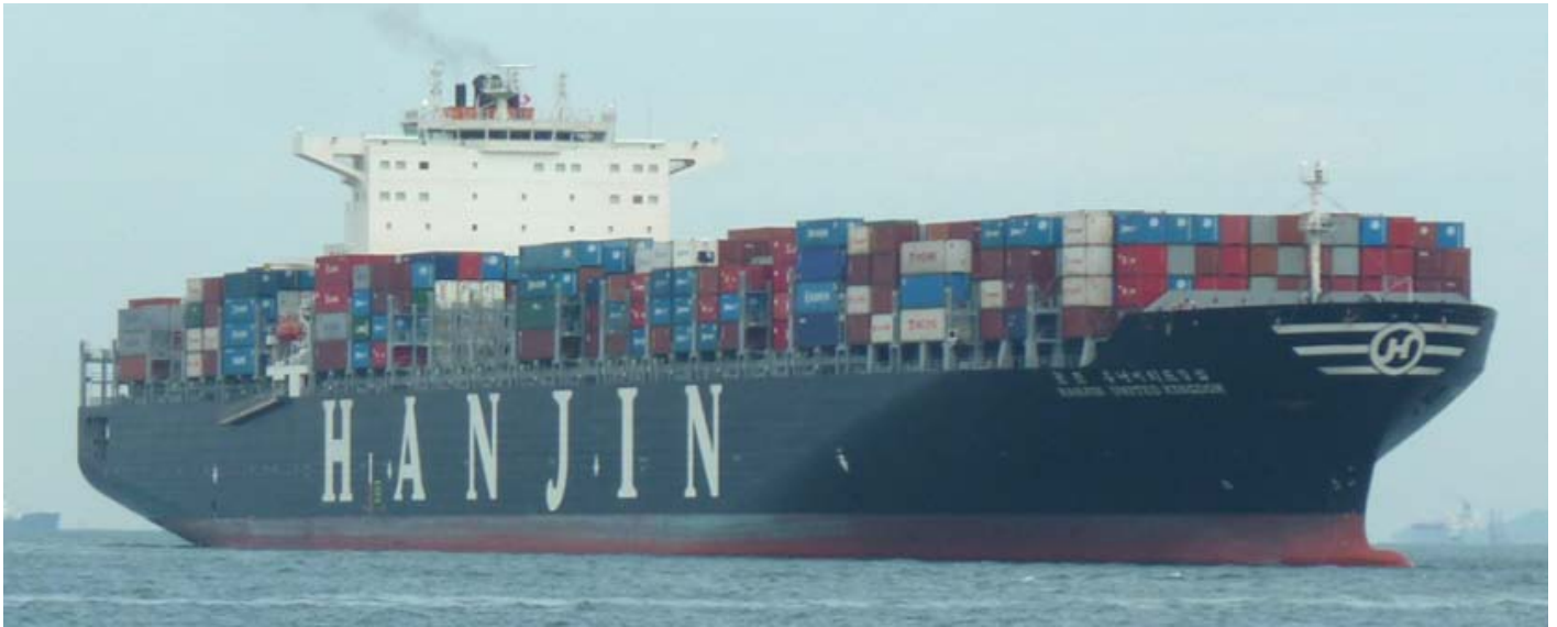
The 2011 delivered 350 mtr long 7200 TEU HANJIN UNITED KINGDOM seen approaching the Pasir Panjang container terminal in Singapore, the 117.000 dwt vessel is built at the Samsung Shipbuilding & Heavy industries Co. Ltd, South Korea and powered by 1 B&W 12K98ME-C engine with an output of 69.900 kW for a top speed of 25,7 knots - Photo : Piet Sinke ©
