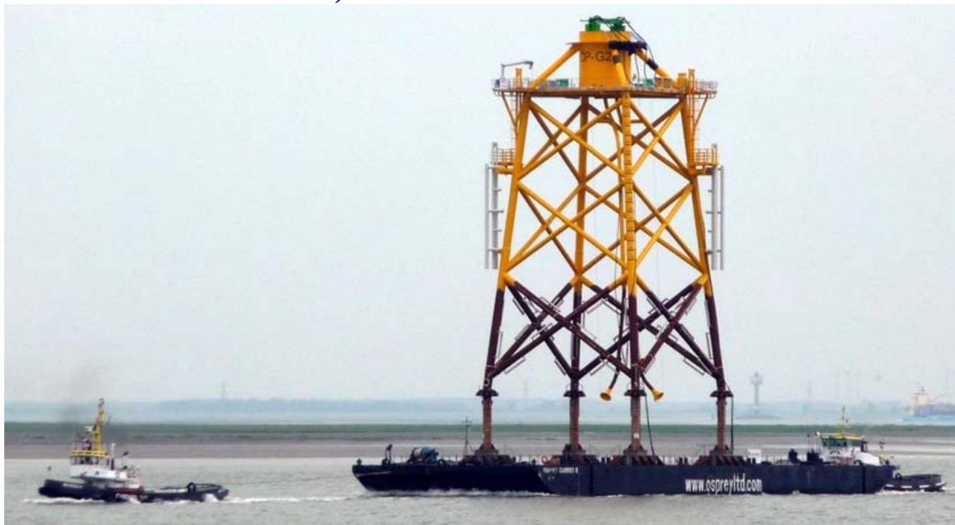
The barge OSPREY CARRIER II loaded with the CP-G2 jacket seen towed by the MULTRATUG 12 and assisted by the KARIN as pusher tug at the Westerscheldt River – Photo : Walter de Groot ©
