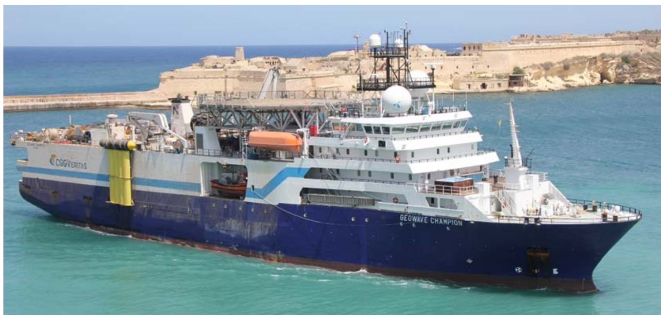
Above seen the 1994 Norwegian built 12 streamer 3D seismic research vessel GEOWAVE CHAMPION entering Grand Harbour, Malta on Thursday 21st July, 2011 for the first time. She was built as the Irish fishing vessel D602 VERONICA of which she was converted in 2007 in Norway as she's now.
