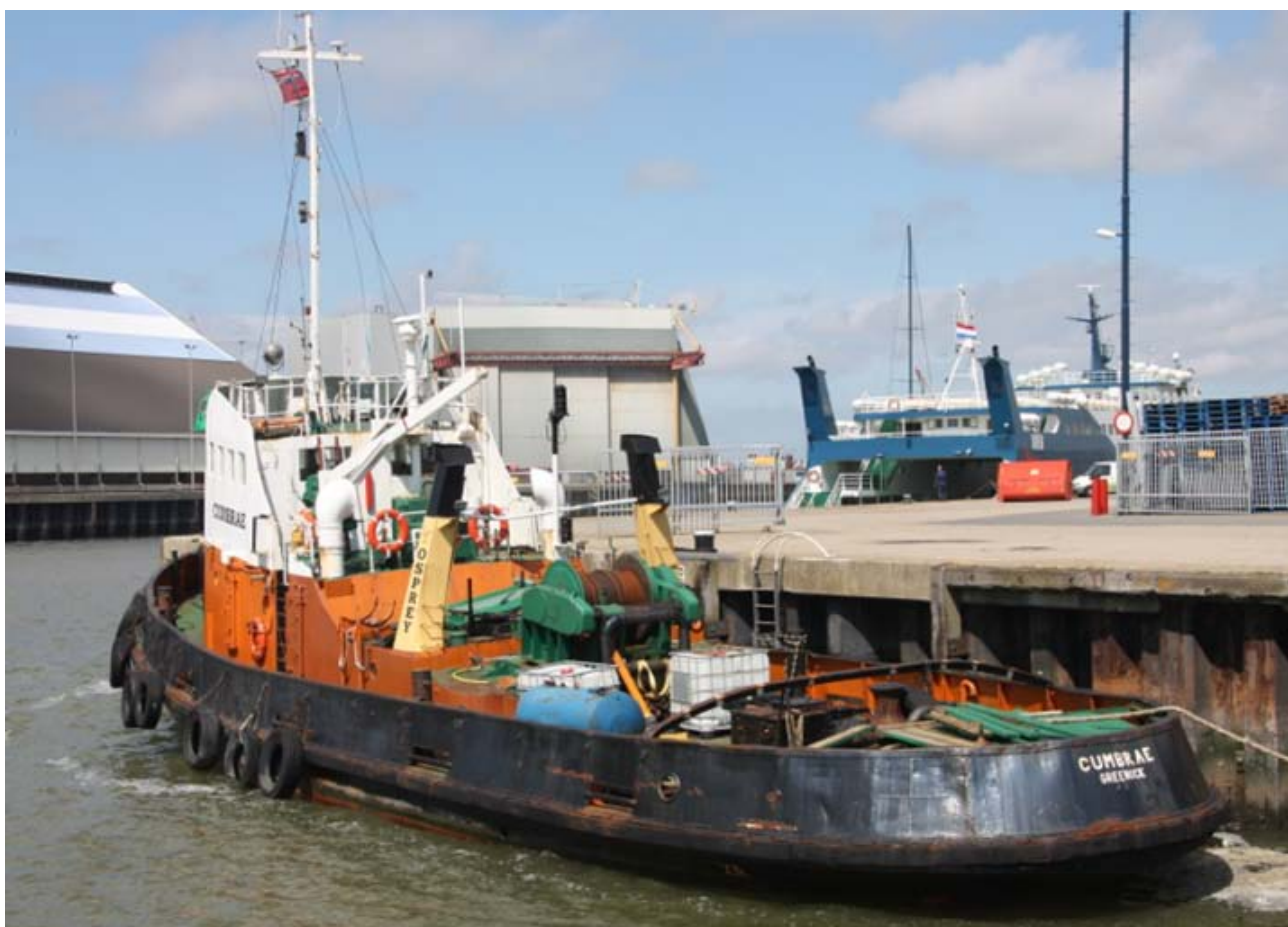
Above seen in the harbour of Harlingen (The Netherlands) the 28,68 m. twin screw motor tug CUMBRAE owned by Osprey Maritime Ltd. delivered as ALSATIAN in 1961 (50 years ago) by Henry Scarr Ltd., Hessele, U.K. Powered by two Blackstone diesel engines with a total output of 970 kW (1.320 HP).
