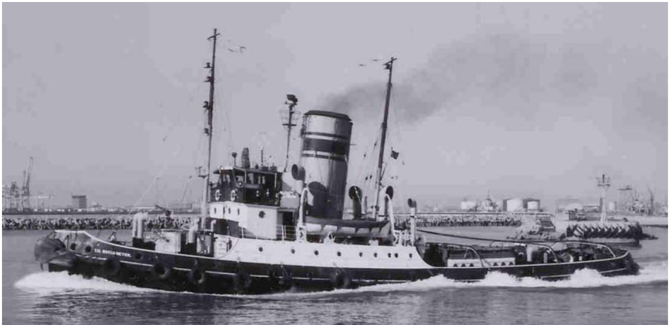
The T.H. WATERMEYER was one of a series of nine coal fired harbour/salvage tugs ordered by the South African Railways and Harbours administration between 1934 and 1939. World War II intervened and delivery of the last two was delayed by about 2 years. The T.H. WATERMEYER arrived in Table Bay, Cape Town, where it spent most of its working life, before being moved to Walvis Bay. A credit to her builders, Inglis of Glasgow, the tug was only retired from service in 1980. Photo: Robert Pabst (c)
