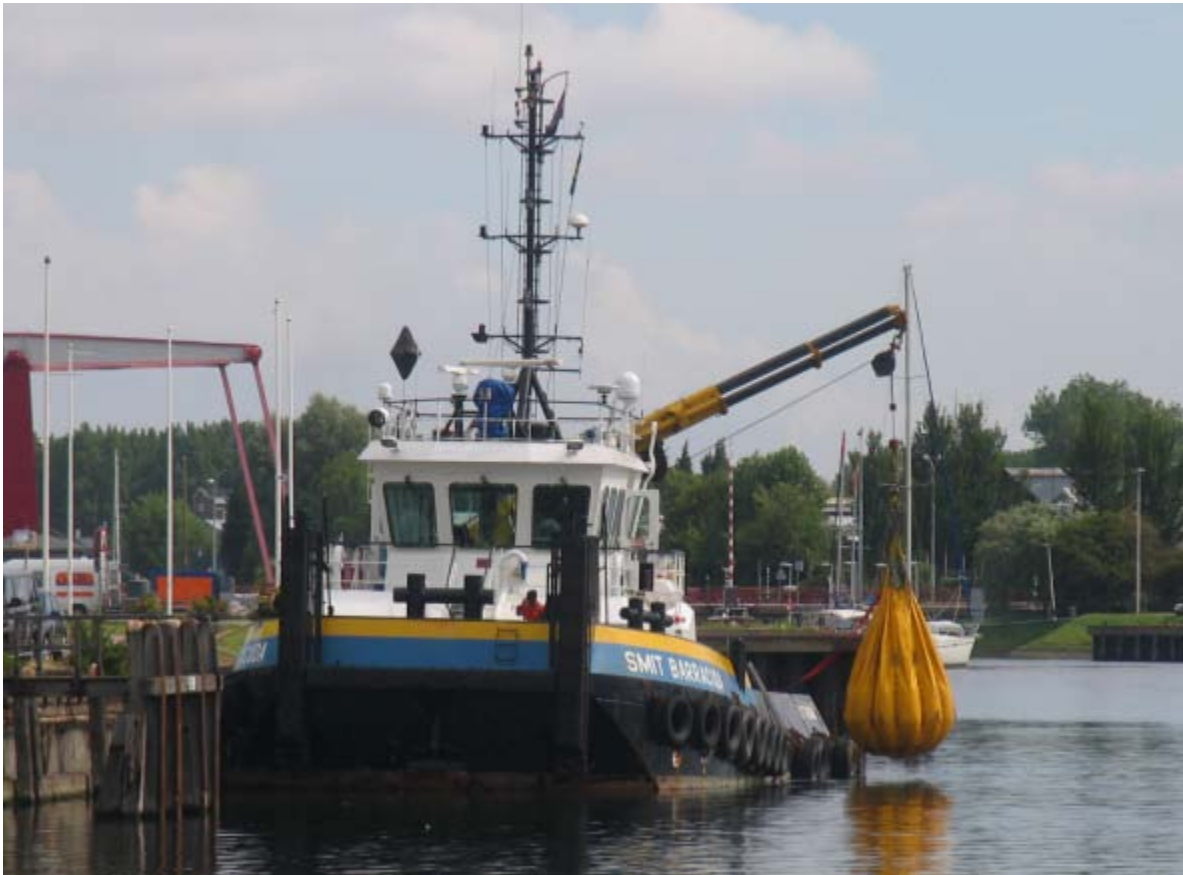
The SMIT BARRACUDA seen conducting a load test on her crane - Photo : Willem Kruit (c)
