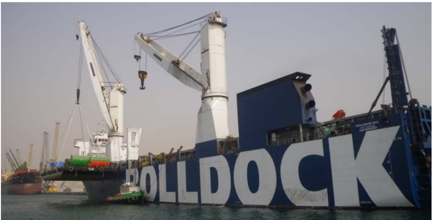
Above seen the loading operation for mv Rolldock Sea's 1st voyage. During the loading operation equipment was loaded by means of flo-flo method and by vessel's both 350 tons cranes. Loading took place in the Arabian Gulf and the vessel will discharge in a Red Sea port. Photo : Jakob Jan Bijlsma (c)
