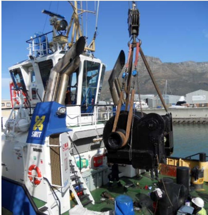
A DMT towing winch seen getting installed on the SMIT MONTSEERAT and SMIT CAYMAN whilst the tugs are berthed in Cape Town - Photo : Lars Herweijer (c)
