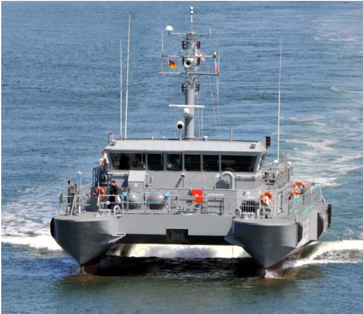
The new patrol-ship SKRUNDA is back in Germany for a check-up at the builder Abeking + Rasmussen in Lemwerder. The SWATH-Boat is the first of five which will built bei A+R and Riga Shipyard until the next years for the Latvian Navy. Photo : Frank Behling (c)
