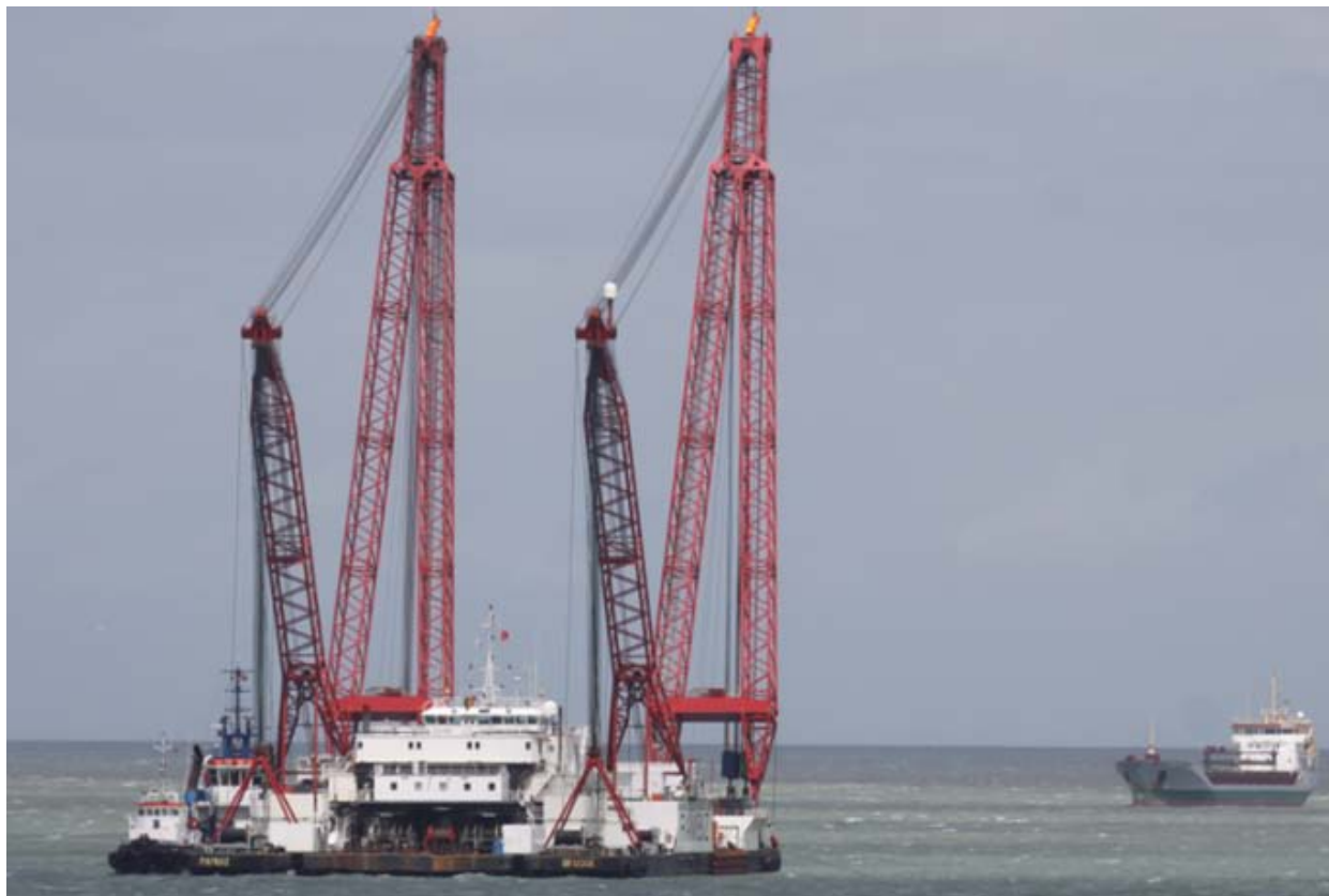
Crane vessel Rambiz anchored in Margate Roads, accompanied by Fairplay 31 and Afon Caradog . Awaiting the opportunity to install two substation topsides at London Array windfarm. - Photo : Peter Barker (c)
