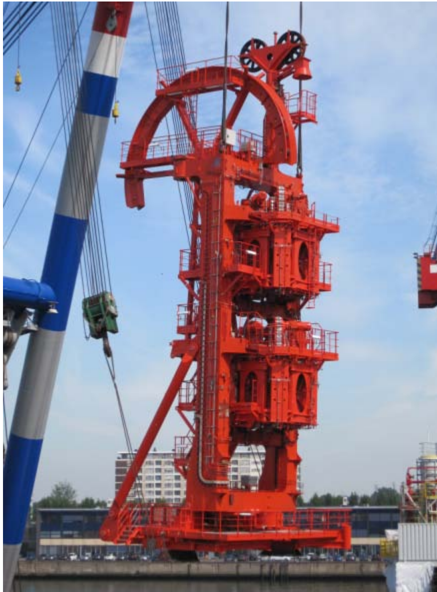
Above seen the Matador 3 , lifting a Huisman made newly build “ 150mT Vertical Lay System ” for EZRA Holding to the test pedestal on the Huisman quay side. Pipelaytower and a 185mT A&R winch will be delivered to EZRA August 2011. Photo : Ronald Krijgsman (c)
