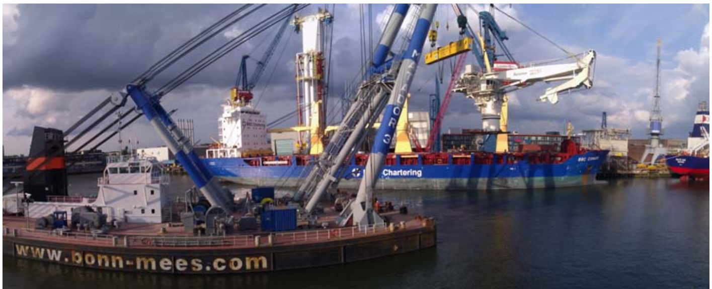
Matador 3 lifting a knuckleboom crane from Huisman yard crane for transport
