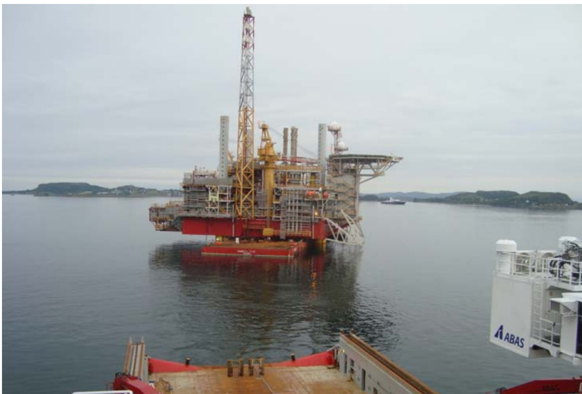
Above seen the YME platform (MOPU) in the Amoyfjord / Stavanger-Norway standby for installation. (Waiting for weather) Normand Prosper connected to the bow (lead tug) and picture is taken from the Far Sapphire connected to the stern. - Photo : Marco Wehrmann – Tow master SBM Offshore/ALP Maritime Services BV ©
