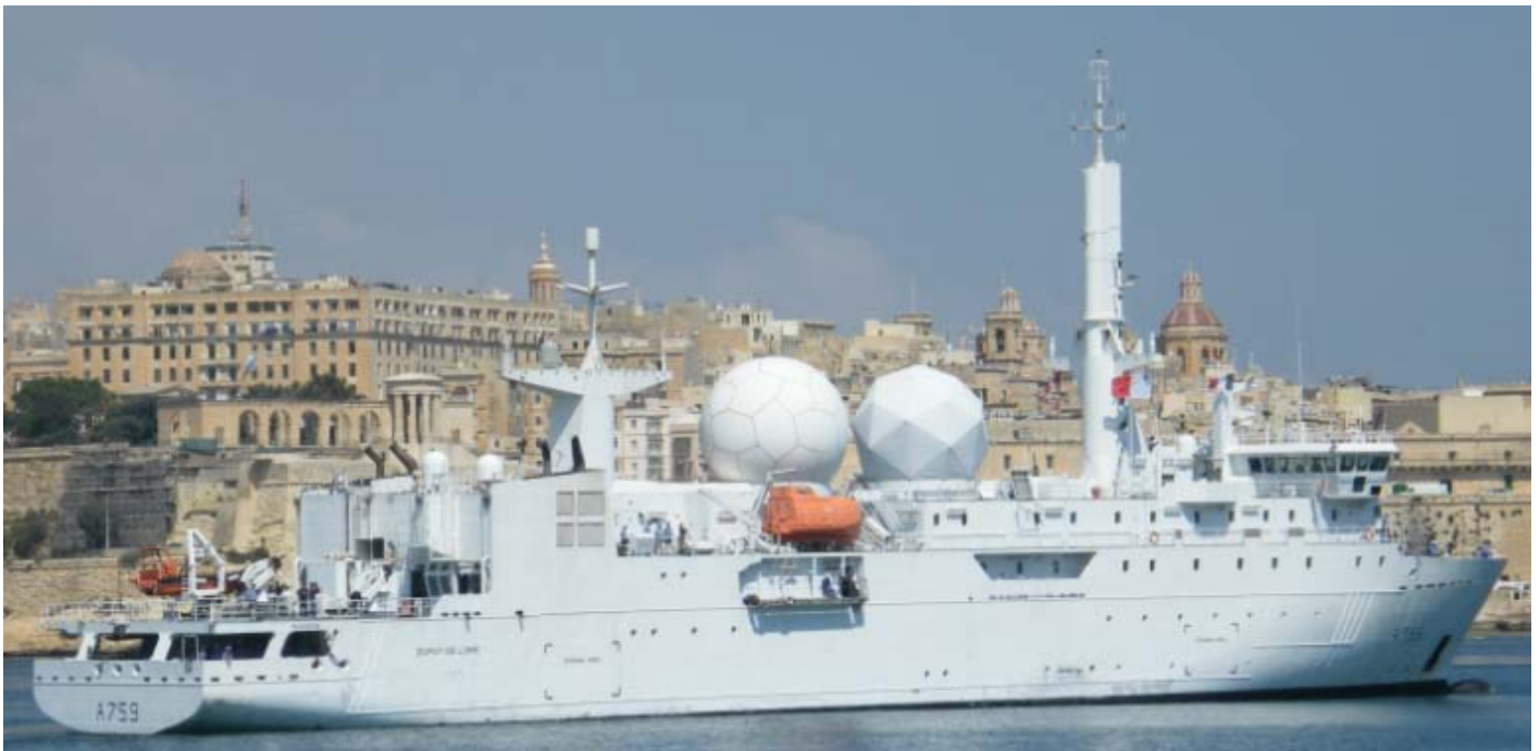
The 2006 commissioned French Navy, Signal and Communication Intelligence Ship, " Dupuy de Lome " ( A759 ). The 101 mtr long vessel is having a Range of 6300 km, of 3100 tons, and is seen above at Bighi Bay, Kalkara, (Malta) with Valletta at the background. Photo : Gejtu Spiteri (c)
