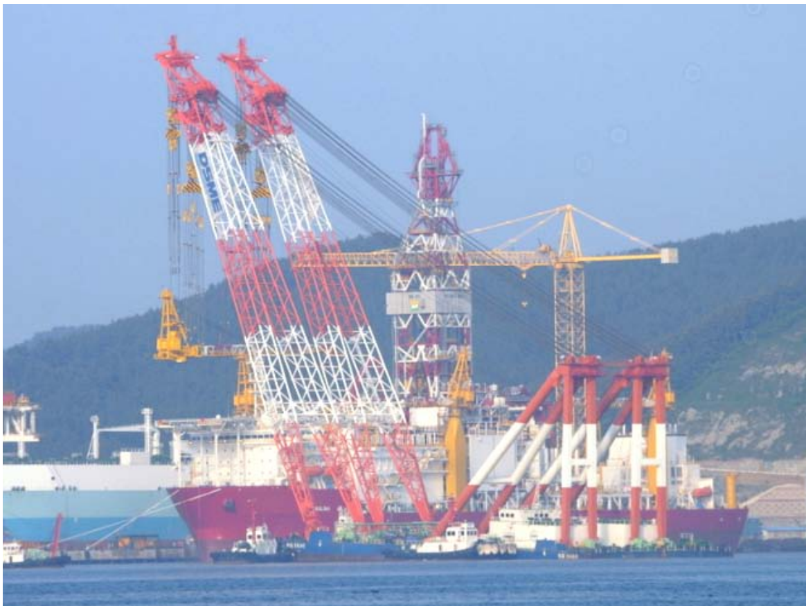
Two large shearlegs seen installing equipment on a new drilling vessel at the DSME shipyard in Busan (Korea)
