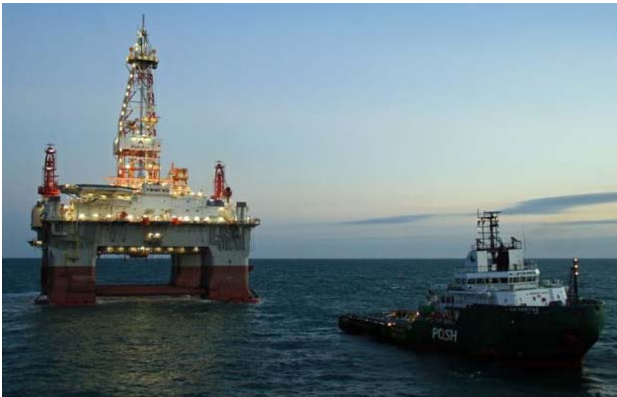
Above seen at Alpha Star standby location off Macae in Brazil. The Salveritas is going in to disconnect and the Maersk Handler and Normand Titan are attaching pre-laid moorings. Rig is in DP mode but Salvanguard still connected for insurance. Photo : Capt Neil Johnston – Master Salvanguard ©
