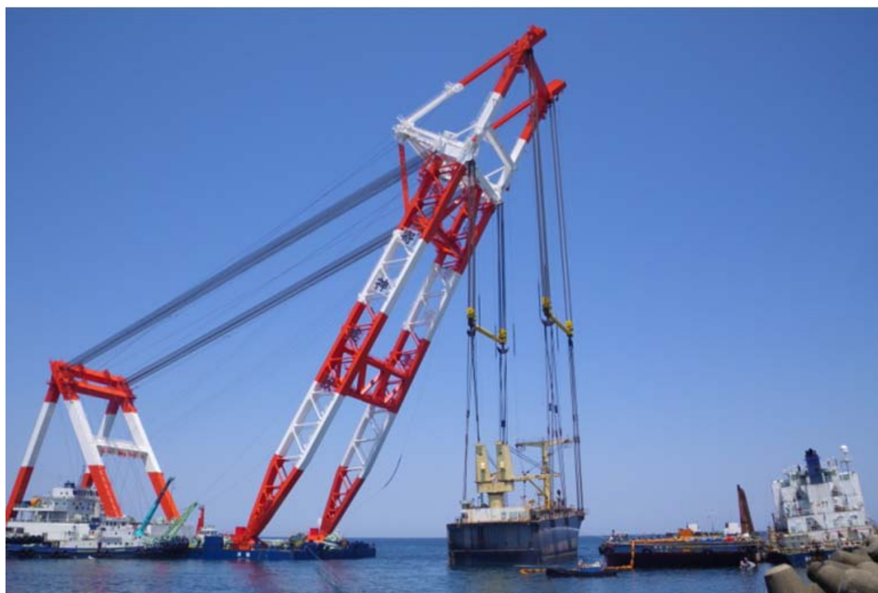
Above seen the wreck removal operation with 4,000ton lifting capacity shearleg "YOSHO" lifting up forward half hull of the wreck ex. "BOHAI CHALLENGE" which went aground on breakwater of Kanazawa Port, Japan in January 2011. Photo : Y.Fukushima ©
