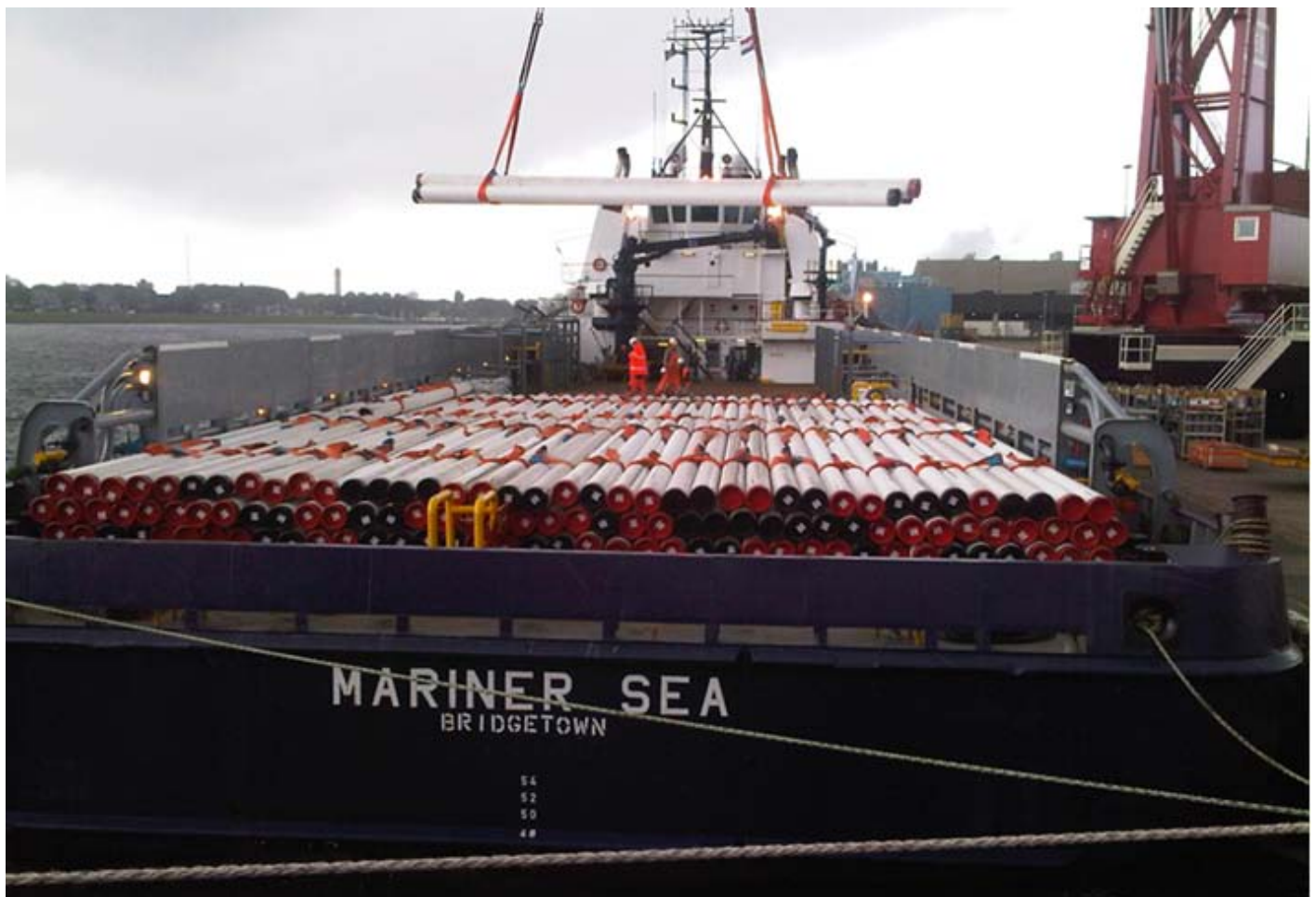
The MARINER SEA seen loading in Velsen Noord 424 pcs of 14" pipe for the Gaz de France project G 16, the Mariner Sea will bring the pipes to the ACERGY FALCON which is laying the pipes. Photo : Geert Woord ©
