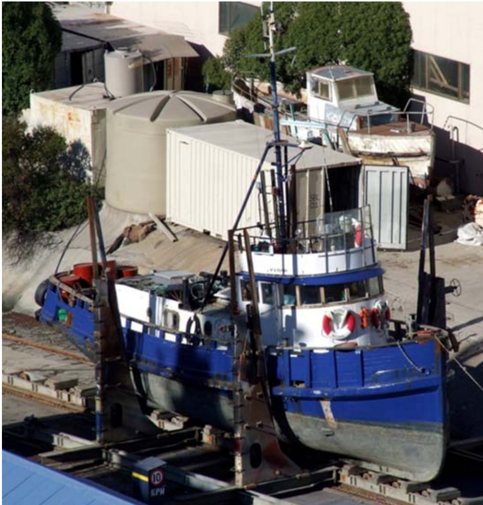
The small wooden hulled tug Rakanui undergoing repairs on the slip at Lyttelton
