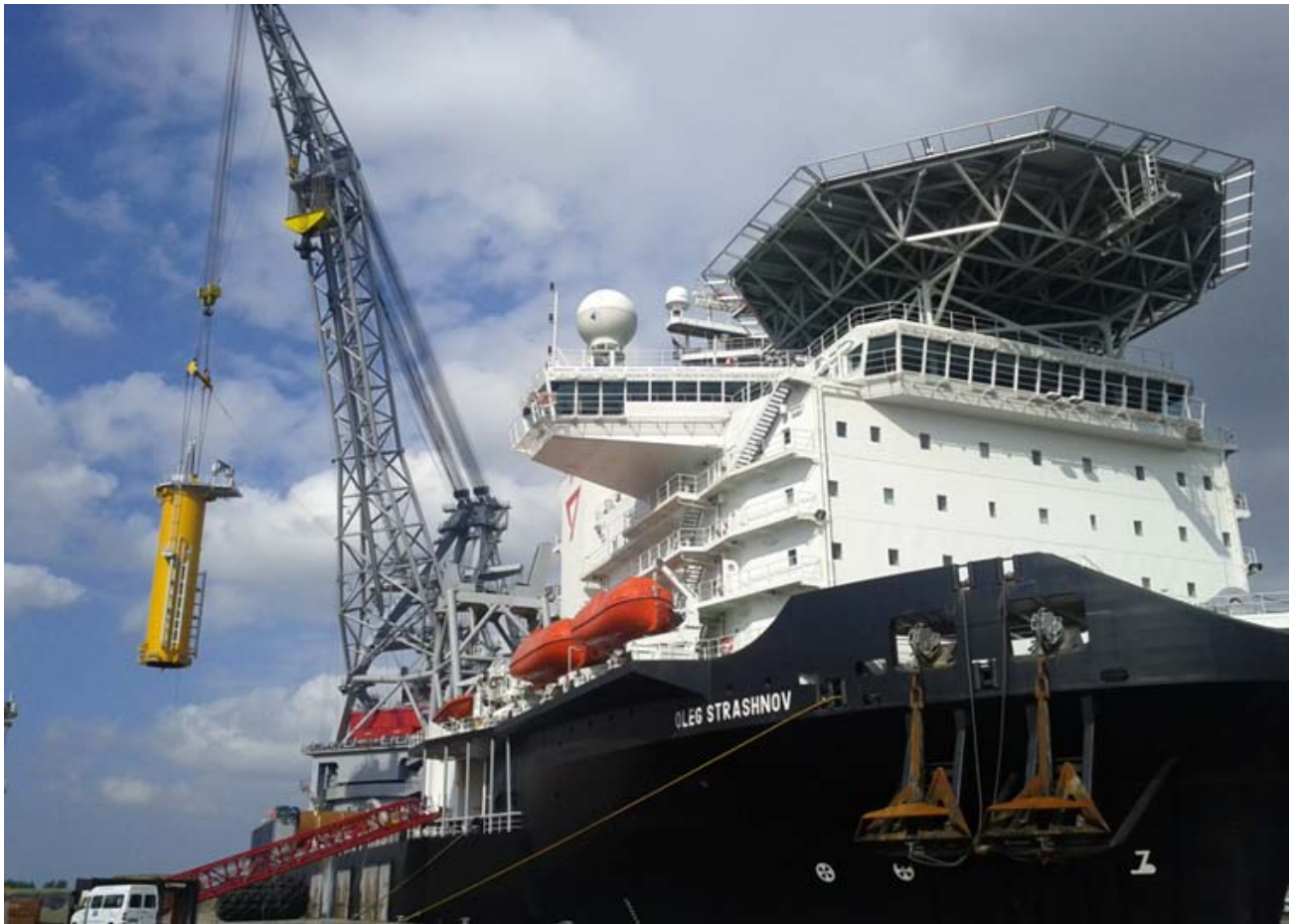
Above seen the " Oleg Strashnov " loading monopoles and currently in the crane Transition Pieces at the Bow Terminal in Vlissingen, items will be installed at the Sheringham Shoal windmill park, which is situated in front of the UK coast. Photo : René Alferink ©
