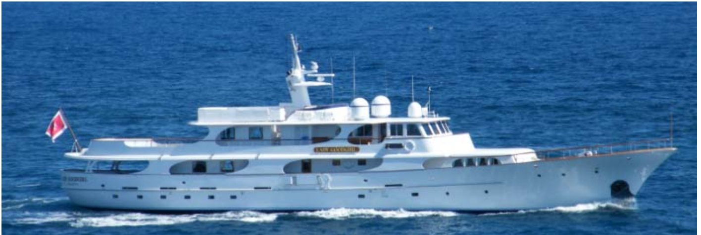
The Classic 1964 built motor yacht " Lady Good Girl ", built by; Hall Russel in Aberdeen. 42.90m in length, 8.00m beam, 316gt, flying the Maltese flag, seen leaving Valletta, Malta, after 7months of modification at Bezzina Ship Yard, Paola, Malta. Photo : Gejtu Spiteri ©
