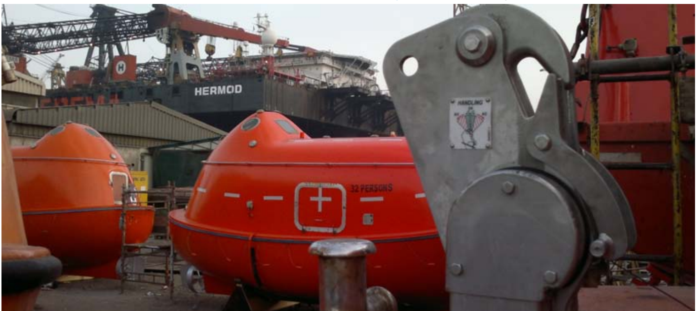
Combined crew of Willem Pot B.V. and Umoe Schat-Harding B.V. re-hooking all lifeboats of Heerema`s "Hermod" with the SeaCure LHR MK II hook system at Dubai dry dock location.
