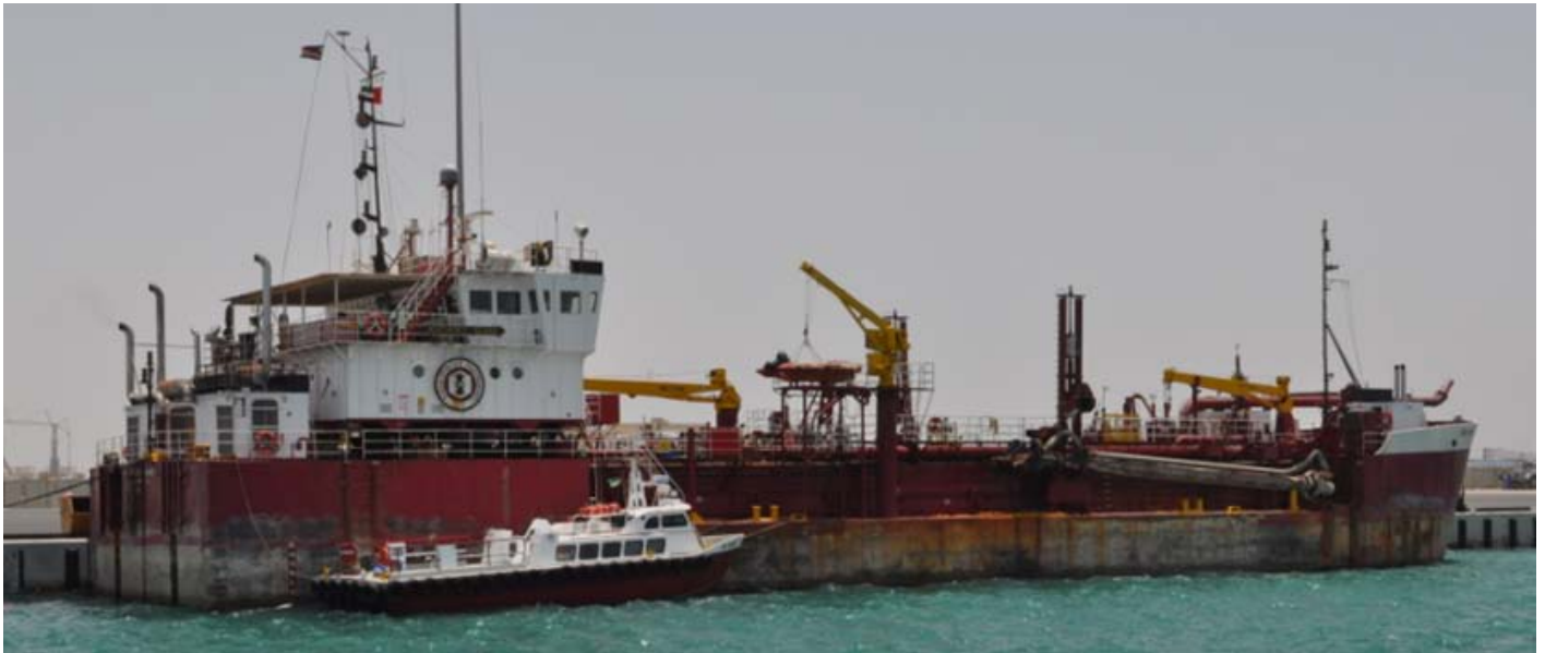
Below seen the Split Hopper Dredger “ Northerly Island ” built in the US 1983, hopper capacity 1652 m2, she was original build for the North American Trailer Company a cooperation between Great Lakes and Ballast Nedam
