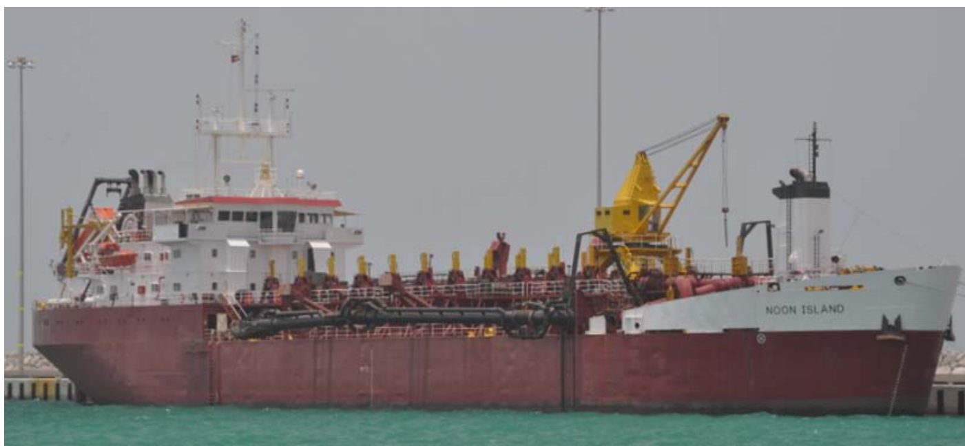
Above seen in Abu Dhabi municipality Port, Hopper Dredger “ Noon Island ” built in 1977 as “ Boa Vista 1 ” for Brazilian owners by IHC Holland with a Hopper capacity of 5600 m3, sold in 2007 to Great Lakes Dredge and Dock Cooperation Photo : Maarten Mostert (c)
