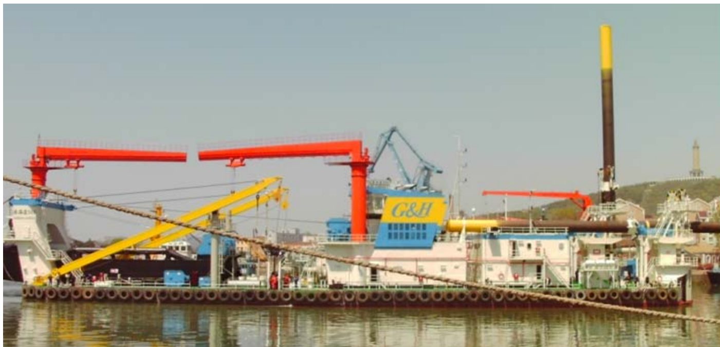
The IHC built Gang Hai Jun 566 finished successfully the water pumping test and returned to the builders to prepare for towing and delivery at Tianjin port later this month - Photo : Cees de Vries ©
