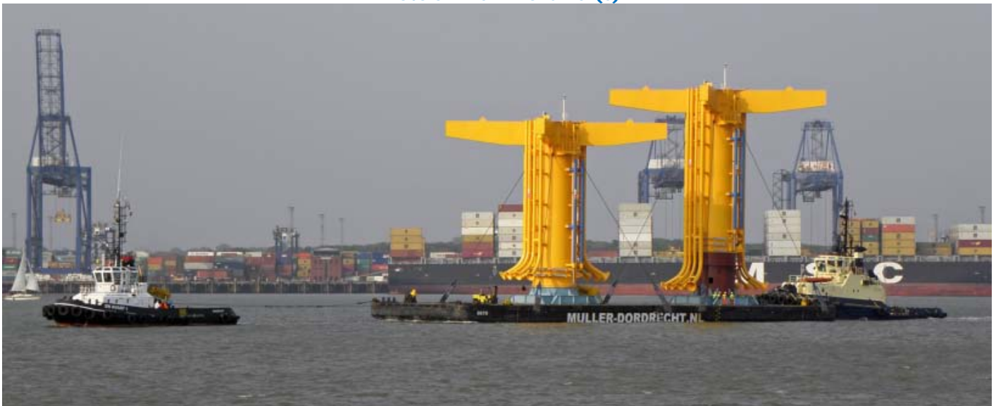
The latest Muller fleet addition EN AVANT 1 (50 ton BP) seen arriving with offshore transition pieces in Harwich, loaded onboard the Muller pontoon 6619 .
