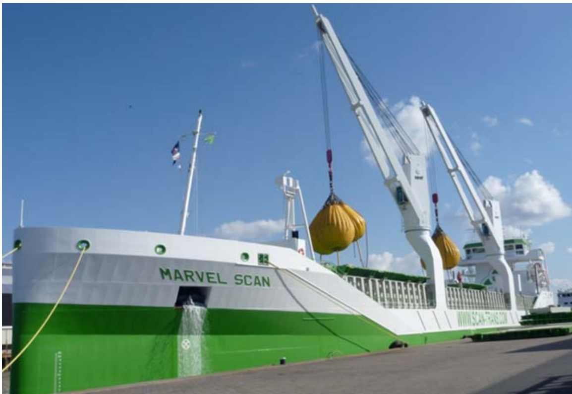
MV Marvel Scan seen performing load tests in Harlingen - Photo : Daniel van der Zwaan ©
