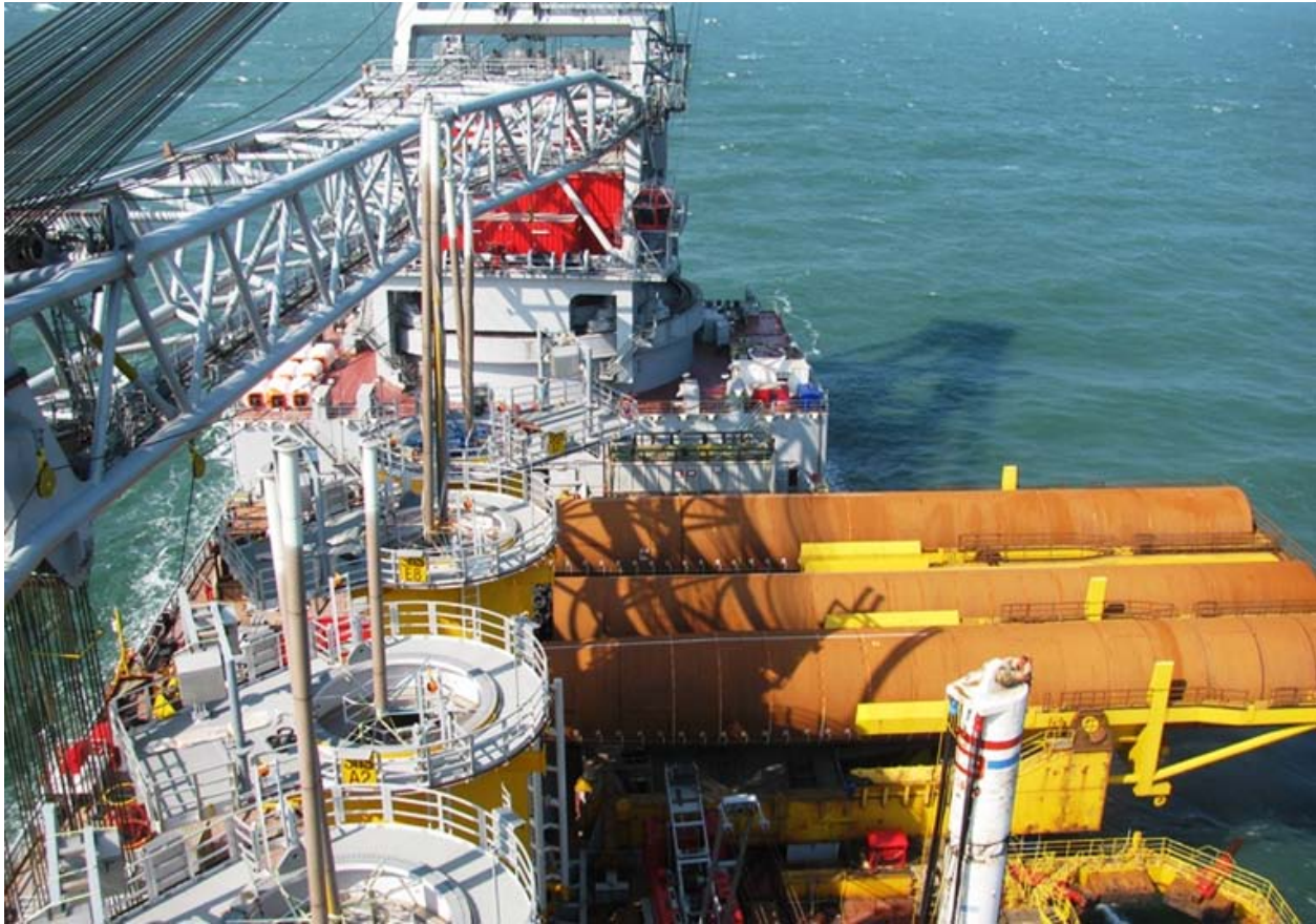
Oleg Strashnov st.by for weather Sheringham Shoal field with a complete full deck of 4 T.P and 3 monopiles. Photo : Adri Haasnoot ©
