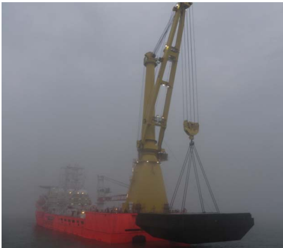
Above seen the Huisman 850t OMC onboard the Caballo Maya – Oceanografia being load tested with 935t at 30m in Zhangzhou, PR of China. Photo : Pepijn Toornstra ©
