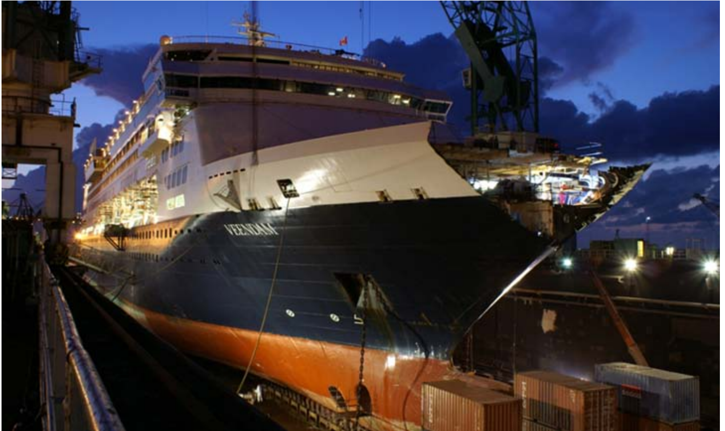
HAL's Veendam received a new "nose" in Bahamas Shipyard after been damaged during heavy seas near the Falklands. Photo's : Veendam Eng.Dept ©
