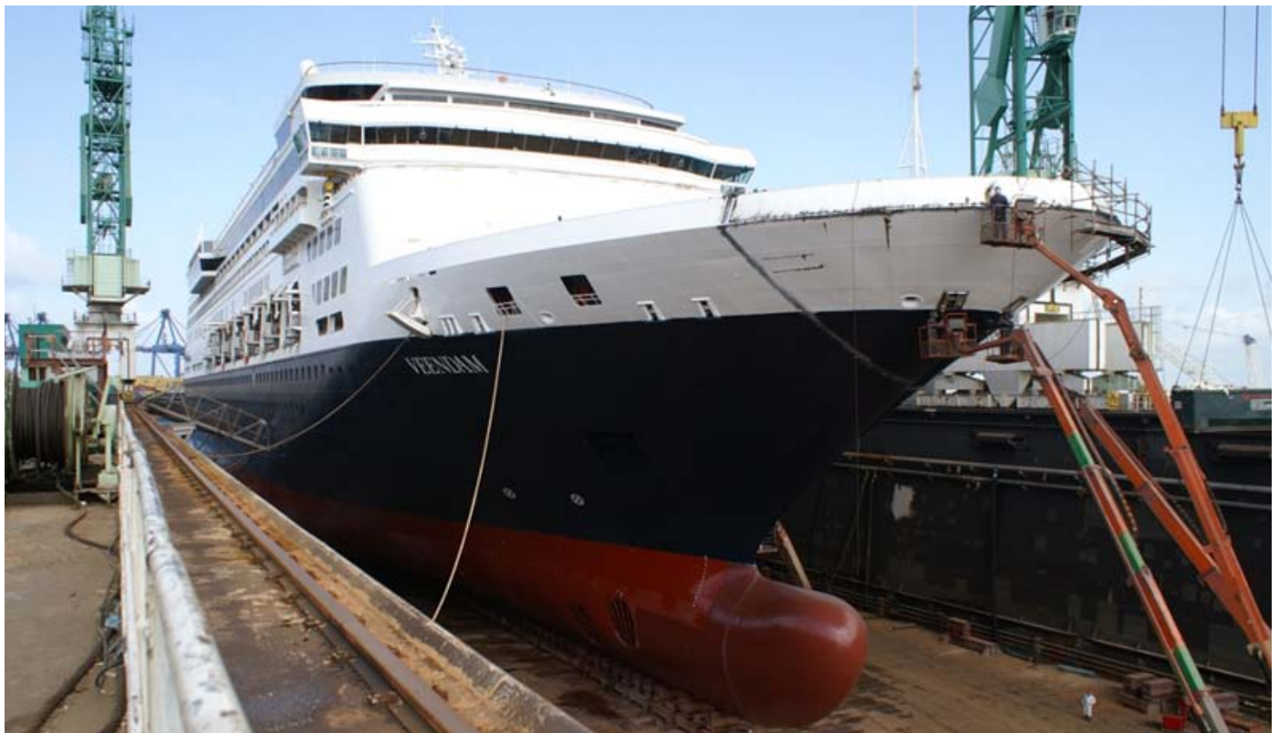
HAL's Veendam received a new "nose" in Bahamas Shipyard after been damaged during heavy seas near the Falklands. Photo's : Veendam Eng.Dept ©
