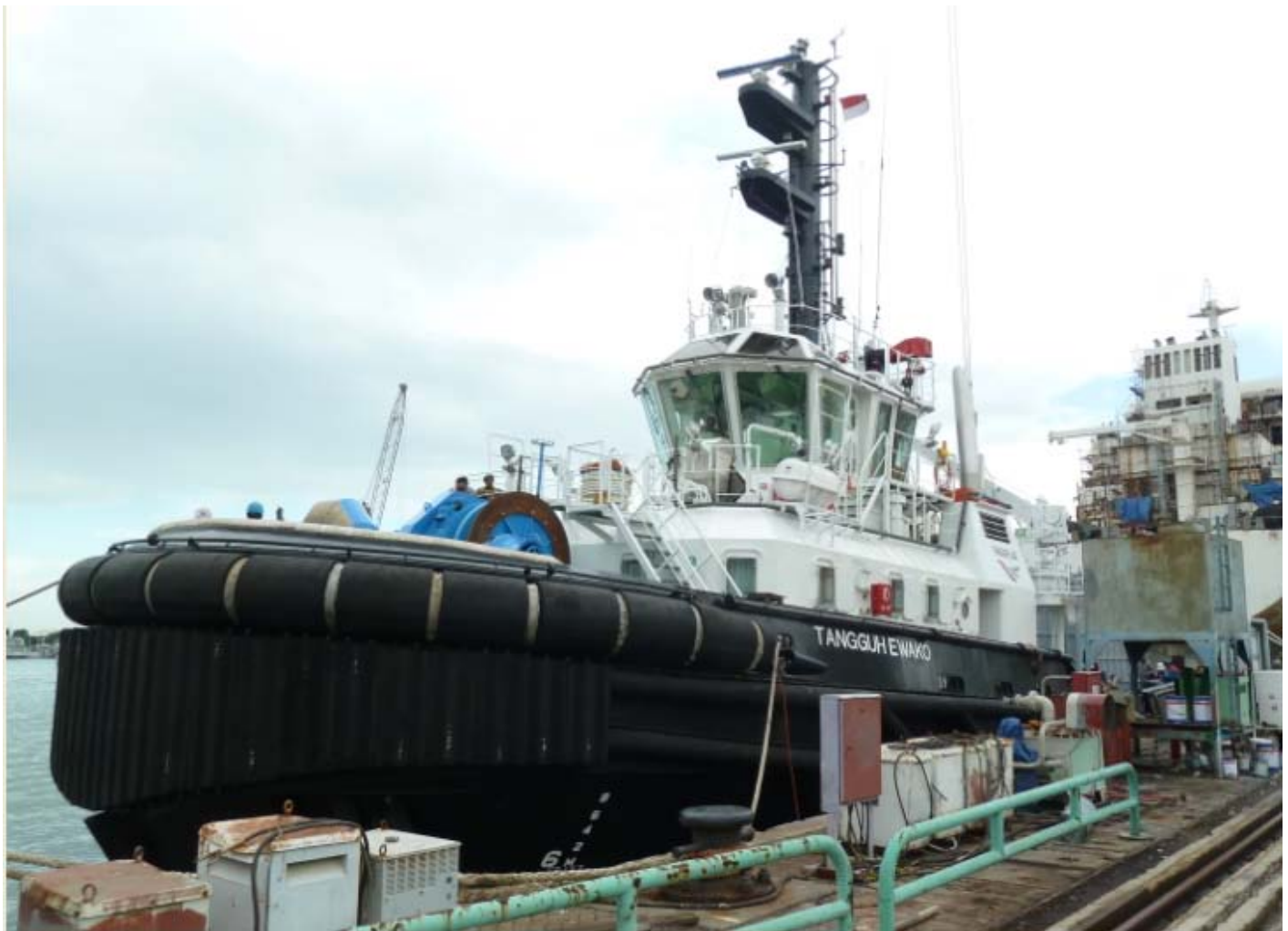
The 4000 bhp/55 ton BP TANGGUH EWAKO seen fitting out at the PT PAL shipyard in Tj Perak (Surabaya)
