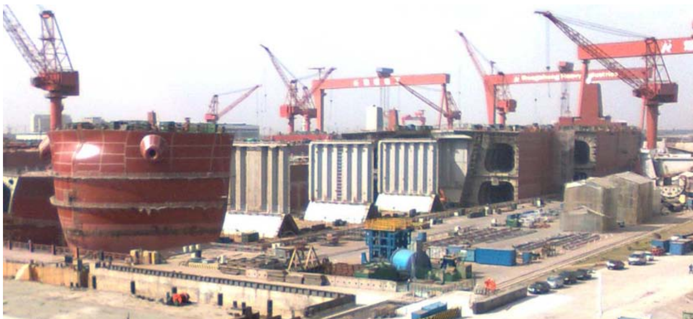
Bulker seen under construction at the Rongsheng Yard in Rugao near Nantong. Photo : Willem Poot ©
