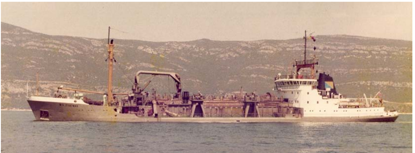
Bos en Kalis hopper dredger W.D Tideway during dredging in Setubal (Portugal) 1978, the W.D Tideway was built by "Blyth Dry-dock and Shipbuilding Company" Blyth in the U.K in 1965 with a hopper capacity of 3004 m3 and a speed fully loaded of 11 knots, she was one of the first hopper dredgers capable to pump her load to the shore by floating pipeline over the bow or by the so called telephone hook fitted behind the foremast. Sold in 1989 to Nigeria and renamed in " MOWA " Photo : Coll. Maarten Mostert
