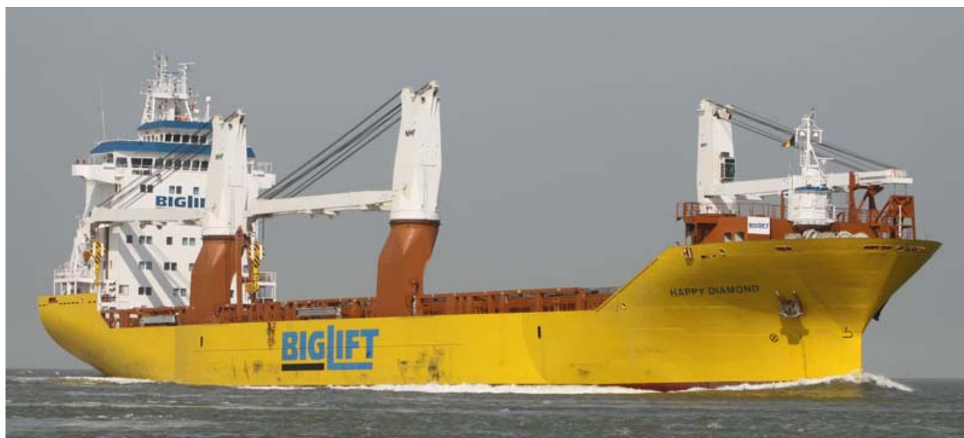
Above seen Biglifts HAPPY DIAMOND seen arriving from the Middle East enroute Antwerp, the vessel is equipped with 2 cranes of 400 ton SWL, furthermore is 1 crane of 120 ton SWL, the HAPPY DIAMOND is the second ship of the D-type, out a series of 5 all built in China
