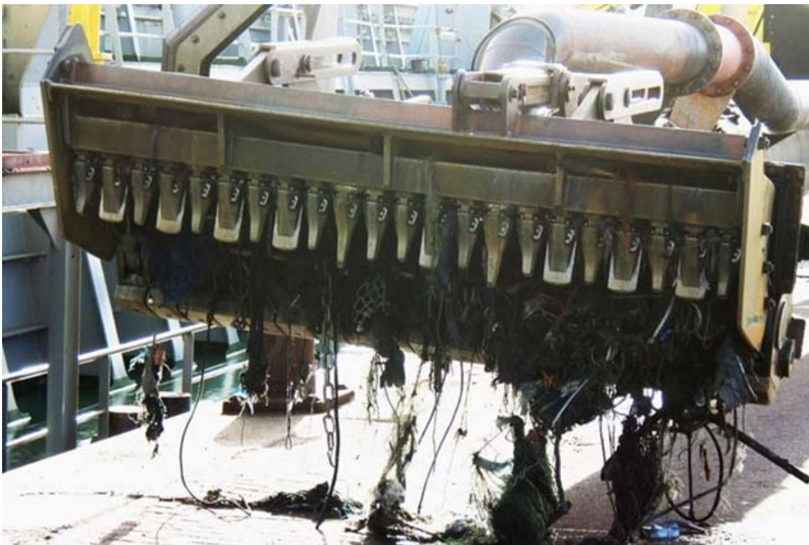
Rubish seen in the suction mouth of the TSHD ELBE which is operating in the port of IJmuiden
