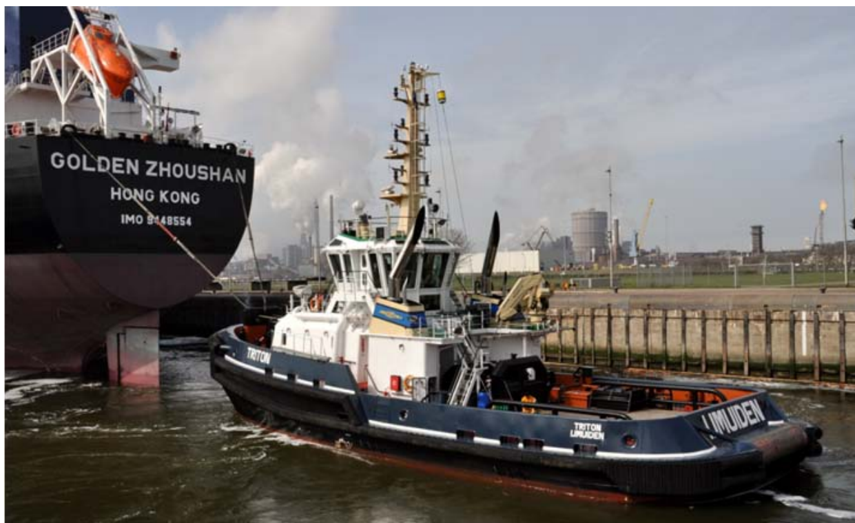
Tug TRITON of ISKES assisting the capesize GOLDEN ZHOUSHAN with a 'Twin Tow Wire configuration' for precise manoeuvring into the IJmuiden locks". Photo : Marcel Coster (c)
