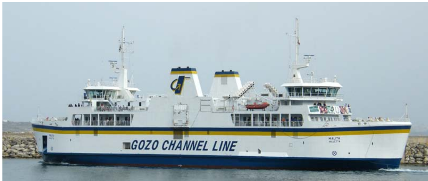
The " MALITA " ferry that can carry 900 passengers + 72 cars on car deck + 66 cars on Hoistable deck
