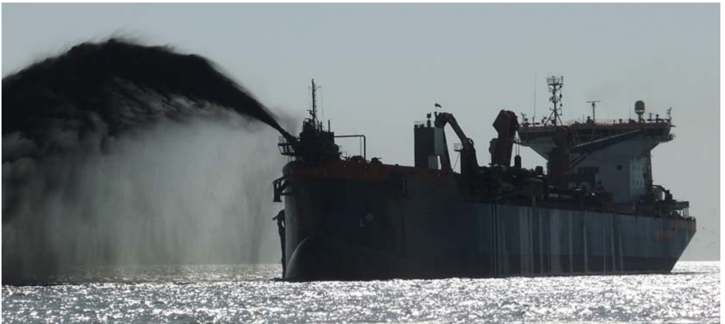
The TSHD HAM 318 is dredging a trench off Iraq at present , above is seen the TSHD during 'Site casten' during this Works 1 dredgie pipe stays on the bottom and the sand is pumped out via rainbow nozzle over the bow
