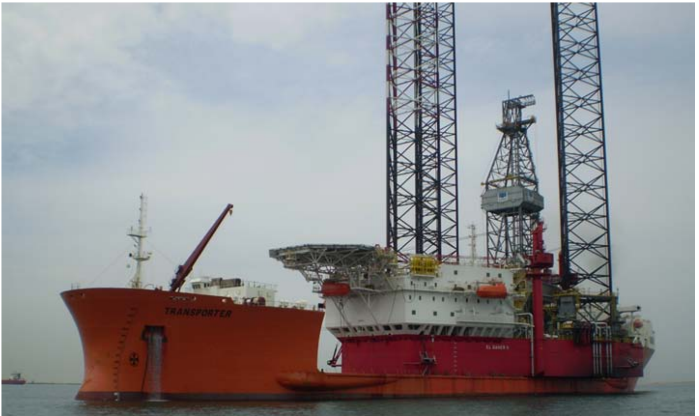
At the West Jurong anchorage in Singapore Dockwise TRANSPORTER loaded the Jack up rig El Qaher 2 Photo's : Anders Bohn Hansen ©
